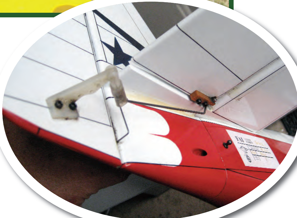
Right: This is a picture of Paul’s Mustang. You can clearly see the wooden pivot point on the elevator. You can also see a ball socket like I have on my 2002 plane. This enables Paul to disable the rudder if he so chooses.
