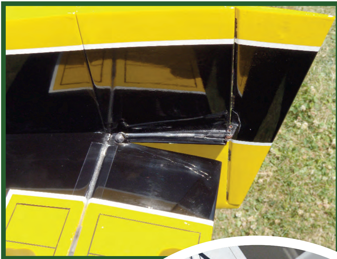
Above: Here is Windy’s setup on his 2009 ship. It is a lot like Kent’s except Windy used a plywood horn on the elevator instead of the ball link inserted into the edge of the elevator.
