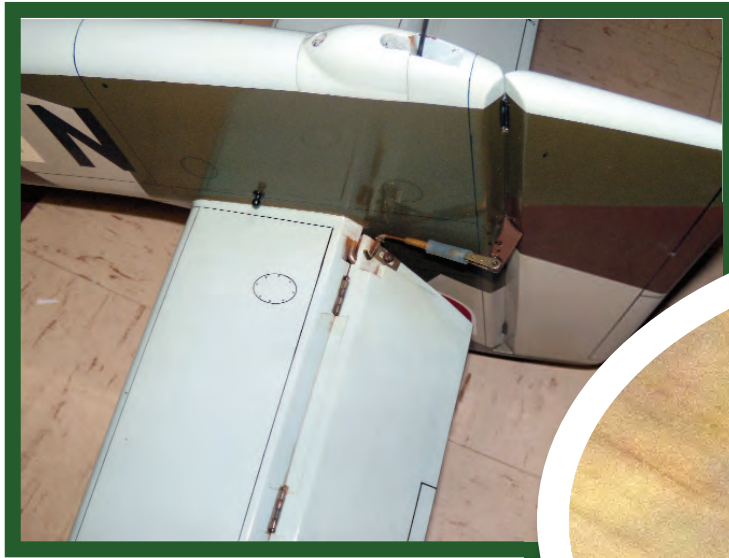
Here is a close up of my 2002 plane rudder. Note the ball socket under the stabilizer toward the front of the plane.
