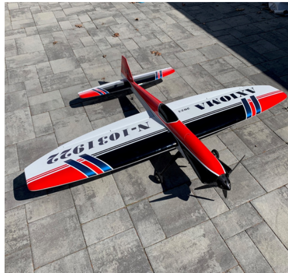
Steven's finished Axioma. He is pretty happy with it. It has a Badass 3515 710kv motor, with an Igor timer and jeti spin ESC flying on Will Power 6S Lithium-ion batteries. All up weight is 66ozs.
