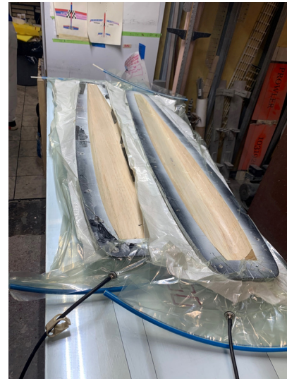
The Axioma fuselage in the vacuum bags.
