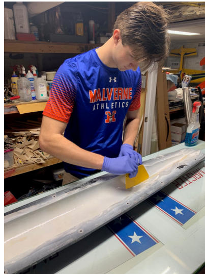
Steven spreading the West resin on the fiberglass.
