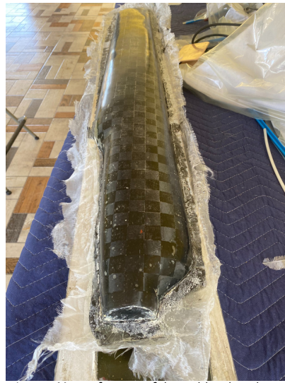
Impact Master fuse out of the mold and ready to clean up. Got to love the carbon pattern.
