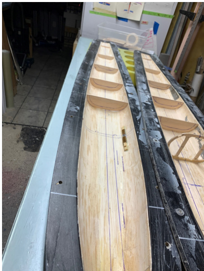
Installing the formers. Building in the molds make it easier to come out in almost perfect alignment.
