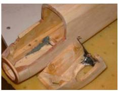
This is a borrowed photo from SSW forum of a spring released cowl holddown. The one I used on the original model failed at the 1968 Nationals and cowl fell off in flight, resulting in disqualification. Use good springs for this.
