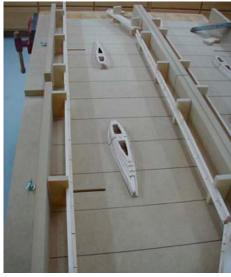
The wing was built in a Tom Morris Millennium Wing Jig, using the Lincoln Log method. To reduce the number of pin holes use Tom's steel weights. Cap-strips are added later.
