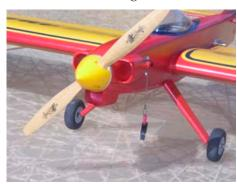
Here is an interesting picture of the front scoops on the Oriental, which are functional. The side scoops cool the battery. The bottom scoop is internally baffled to allow good cooling to the outer rotating shell of the AXI motor. Air from this scoop is directed up and over the motor. The air then goes down behind the baffle and exits at the Rear of the scoop. This baffle clears the bottom half of the motor by a mere .01 to .02 inches. There is also an exit for
