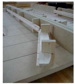
This shows the built up trailing edge stock at the tip of wing in the Lincoln Log building jig.
