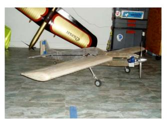
I used Brodak primer with my Harbor Freight HVLP gun and am very impressed with the primer and the gun. I waited 24 hours and sanded the primer down with 3M 220 and 400 open coat paper to the point that very little of the primer was left. I did the same with the flaps, rudder, and elevators. The primer fills nicely, sands effortlessly and the HVLP gun puts it on with minimal wastage.
