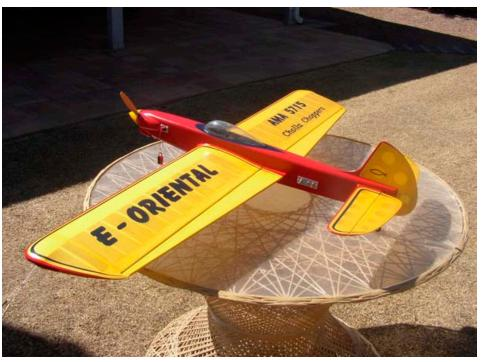
Glen meticulously built this airplane to be very light - that always means very careful selection of balsa, adhesives, and finishing. The fuselage
