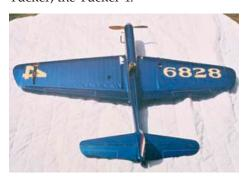
As can be seen from the pictures the original model was in obvious need of some tender loving care. The engine was frozen solid, but the overall structure was in very solid condition. The original had a Fox 35 with no muffler and a ½" shaft extension. The model has an I-beam wing structure and weighed 1100 grams (38.8 oz).
