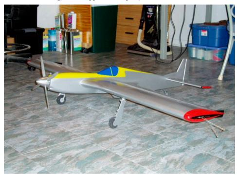
To complete the effect, I used Rapidographic India ink pins for panel lines to add a touch of realism. I made color decals of the lettering on the aircraft via computer using MS PowerPoint and a laser color printer. The decals were applied with Micro-Set & Sol and then sealed with a dry coat of 50/50 clear dope along with the ink lines.
