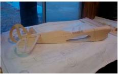
Fuselage with tail feathers cowl and cockpit, Formers for cockpit cover are cut from 1/8 5ply plywood. I have used 1/8 aluminum tubing for these and works quite well.
