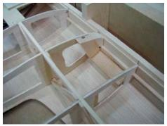
Landing gear blocks made from spruce. Note the 1/16 balsa added at leading edge to support the 1/16 inch sheeting. False ribs from 1/16 ply at both ends of gear block.
