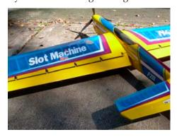
This flap application accomplished by just making the hinge point for the flaps to be inside the trailing edge of the wing. (Hence referred to as a Hofacker Hinge or "Hofflappers") The Hoflapper Hinge is unique, at least for slotted flaps, in that it works in a symmetrical fashion. In other words, you get the same geometry for up as well as down flap angles, and the slot effect is present for both directions.
