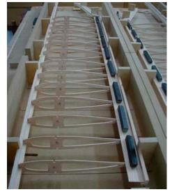
The wing was built in a Tom Morris Millennium Wing Jig, using the Lincoln Log method. To reduce the number of pin holes use Tom's steel weights. Cap-strips are added later.
