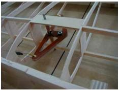
Figure 1 Bellcrank mounting. Original had a 3 inch Veco bellcrank.
