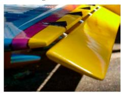
In other words, a blunt wing trailing edge and a sharper flap leading edge could maybe keep the slot effect dormant until some predetermined deflection before it is unleashed. Or, a sharp wing trailing edge and a blunt flap leading edge might effect a gradual turn on of the slot effect. This aspect of the application needs some work.
