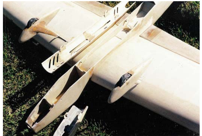
Molded belly shell and cowl removed
