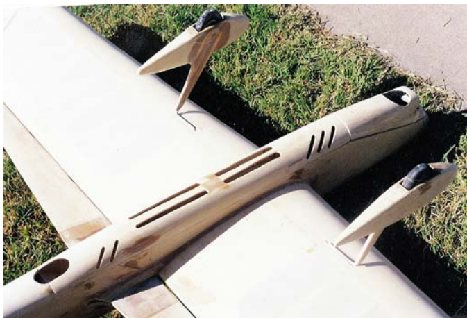
Special Effects' under side, belly shell and cowl in place
