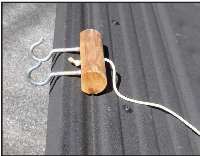
The handle nest was made from a piece of handrail wood stock and two J-hooks with threaded ends.
