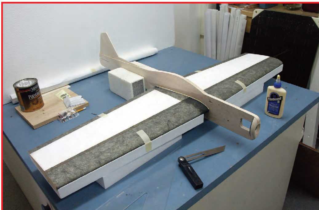
The Joe Nall Cadet wings and fuselages were assembled in a fixture that was made up from the lower wing cradle halves. Note that there is no balsa sheeting on the foam cores. Two-tenths ounce per square yard carbon fiber, attached with water-thinned Titebond glue, was used to strengthen critical areas of the wing. Hunt photo.
