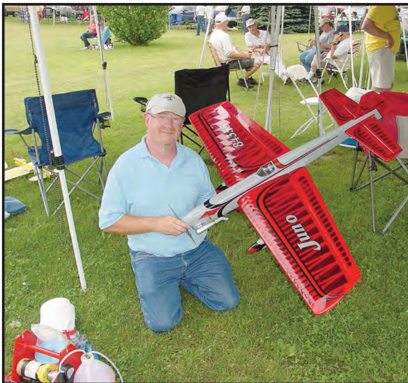
Bruce Jennings's Bill Werwage-designed Juno is absolutely gorgeous! Bruce covered the I-Beam wing with transparent MonoKote and painted the fuselage with automotive paint. Bruce flew this ship in the Advanced class to a well-deserved fourth place. Cralley photo.
