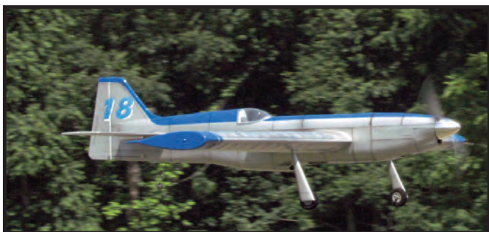
Another veteran model at Brodak's was Tim Stagg's electric-powered Tsunami. Tim's ship utilizes a Power 32 motor a Hubin timer system and 2,800 mAh, five-cell batteries. Here's another ship that displays fine surface detailing. Aud photo.
