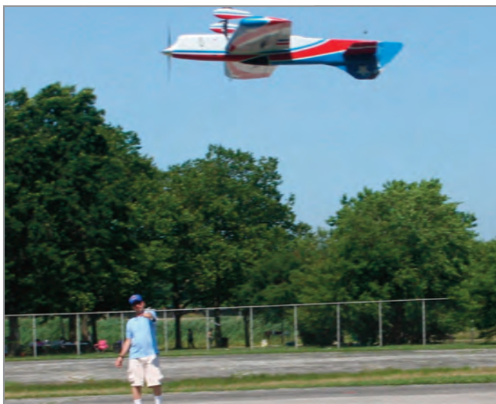
Will DeMauro managed to get in a few practice flights in preparation for the Nats at the fun-fly. His SV-22 is powered by a Scorpion electric motor. Ron Heckler photo.
