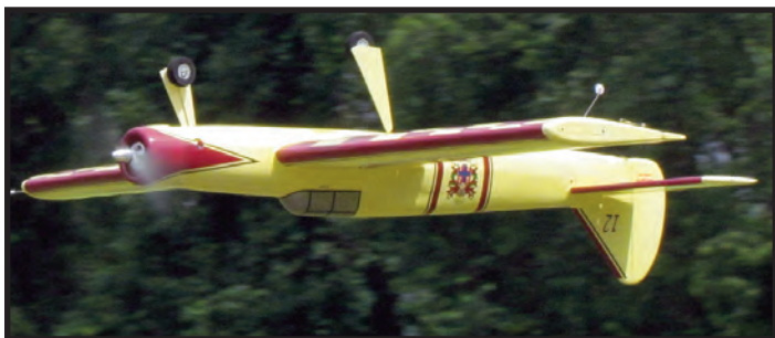
Scott Reynolds' original-design Voltaire features a ring cowl. This very neatly built ship is electric powered and features molded construction. Aud photo.
