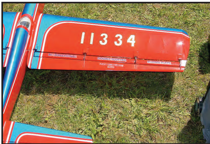
Wes Dick was sitting in his living room contemplating the Venetian blinds one day when it dawned on him that they could be made into flaps! Seriously, his Bi-Directional, Double-Slotted, Blown Flaps seem to work very well. Cralley photo.
