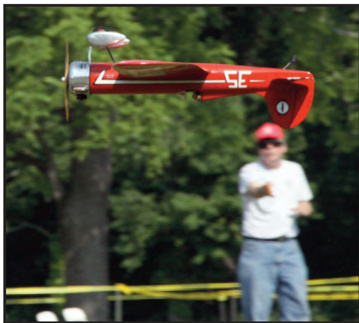
Red Reinhardt's Galloping Comedian is the weapon of choice for OTS competition for Dan Banjock. Dan hand-spun the aluminum cowling for this model and it is a work of art, as is the rest of the model. Dan uses the ubiquitous Fox .35 for power in this model. Hubin photo.
