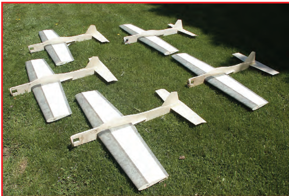
Here are the five Joe Nall Cadet assembled airframes ready for a thin coat of polyurethane clear on the wood parts and then installation of the motor, battery and landing gear. The five models were built by a very dedicated crew in less than a month! Plans will soon be available for this model through PAMPA Plans Service. Hunt photo.
