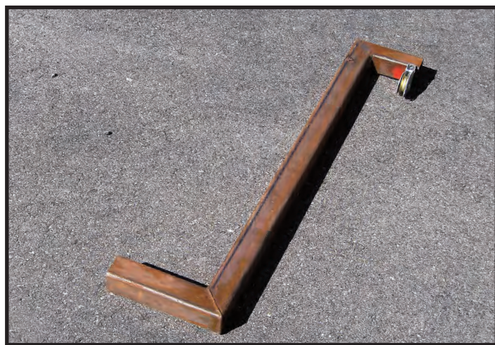
A 4-foot piece of square steel tubing was cut at a 45° angle on the ends, rotated, and welded to make a shape similar to an elongated "Z" without the slant.
