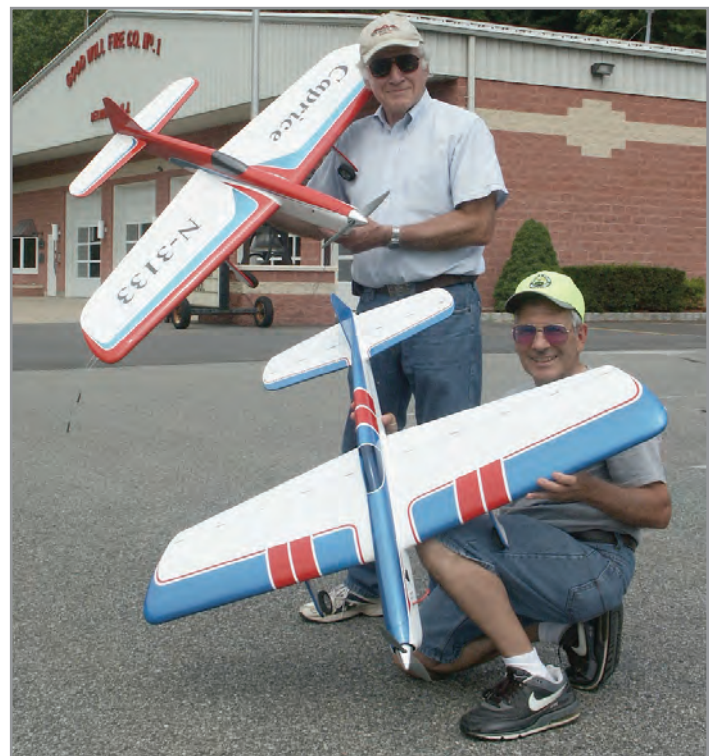
Rich Giacobone (standing) and Frank Imbriaco are justifiably proud of their electric-powered Caprices. They are each powered by E-Flight Power 15 motors running on Hyperion 2,500 mAh 4S batteries, Will Hubin timers, and Castle Creation ESCs.
