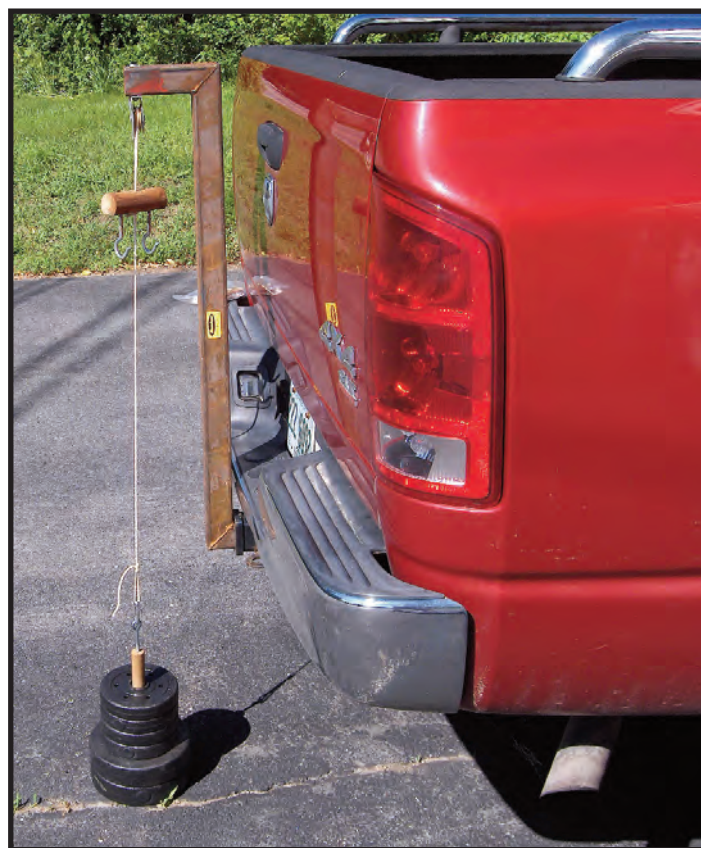
The weight-mounting rod can accommodate 25 pounds of weight.
