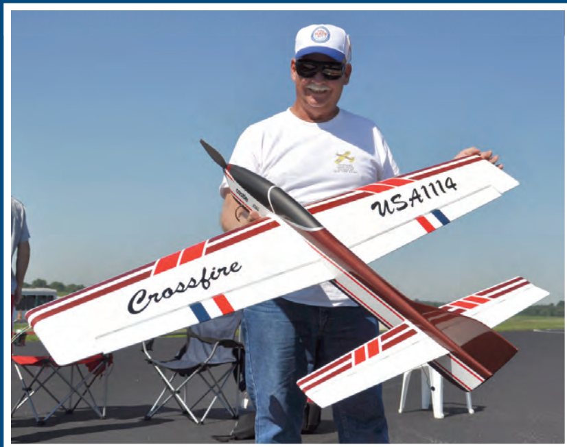
Here's Bob Hunt at the 2011 Nats with his new, electric powered, Crossfire Extreme. The model features a Masterlite foam wing that was cut and covered with the flaps integral to the airfoil. The flaps were then separated and framed with balsa. Photo by Gene Martine.
