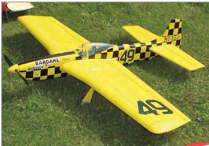
Mike Palko won Expert Stunt at the 2012 Jim Cole Memorial contest. He finished ahead of Bob Hunt and Dan Banjock in a tightly fought, fun contest. Here is his exquisite, Bob Hunt designed, P-51 Mustang. It is powered by a Steve Neu 1907/2Y electric ORK (Outrunner Killer) motor.
