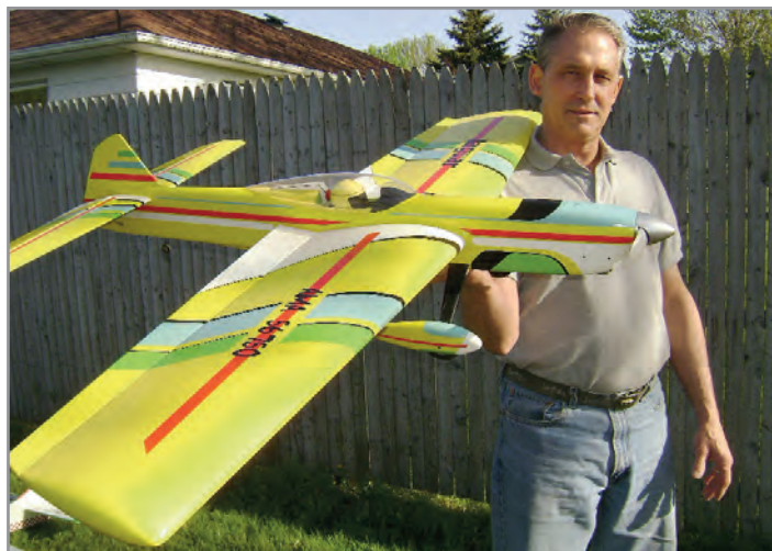
Here's another look at Dave's Jaguar. It is powered by an LA .46 and features a balsa sheeted foam wing, stab, and elevators. It weighs a svelte 55 ounces ready to fly!
