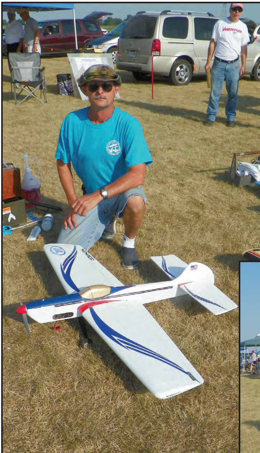
Above: Bob Hudak flew this very clean, electric-powered Legacy to a second place finish in Open Intermediate. The power train consisted of an Emax 2826 motor, a Castle Creations Ice Lite 50 ESC, a Hubin FM-9 timer and ThunderPower 4S 2700 mAh batteries.
