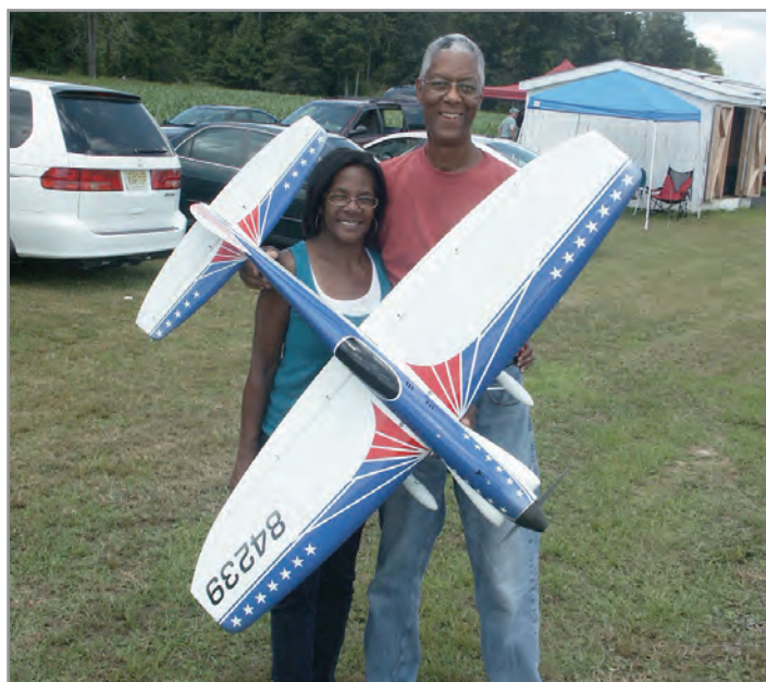
Linheart and Patricia Smith, from Bedham, MA, pose with Linheart's electric powered Yatsenko Shark. With this model Linheart placed first in Advanced at the Hazleton, Pennsylvania contest. It's powered by a Plettenburg Orbit 28 series motor and a 5s 2700 mAh ThunderPower battery. A very nice combination!
