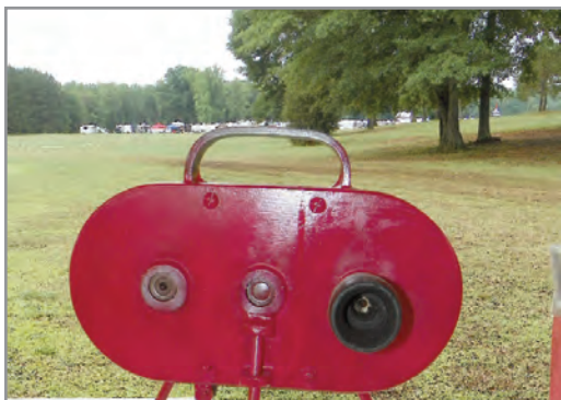
An unknown person brought an inertia/hand cranked starter for speed models to the Joe Nall. This was probably used in the 1950s and '60s to safely crank speedsters.
