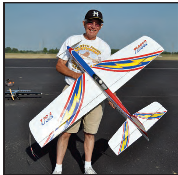
Right: Mike Haverly-built Norm Whittle's E-Sultan for this year's Nats. It is powered by an E-flite Power 32 motor controlled by a Castle Creations Phoenix 60 ESC and a Hubin FM-9R timer.
