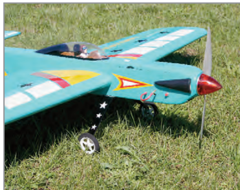
In this photo you can see the safety connection that completes the circuit from the battery to the ESC, the start button, and the functional air scoops.
