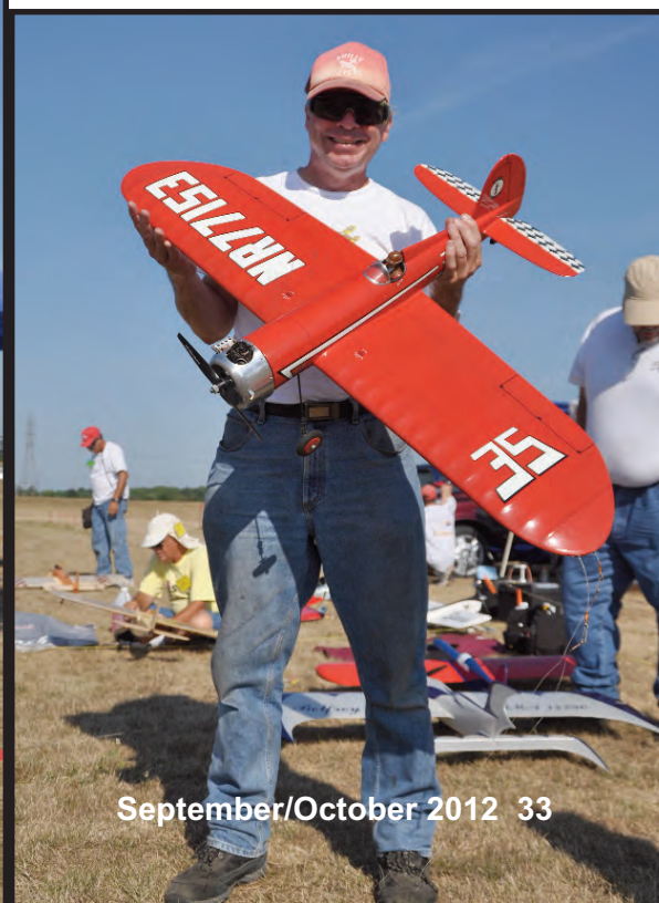
Below: This Harold "Red" Reinhardt-designed Galloping Comedian was built and flown by Dan Banjock. It is powered by a Fox 35 and features a custom, spun-aluminum cowl by Dan.
