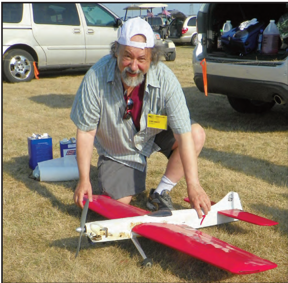
Left: Dennis Moritz, of the Philly Flyers, flew this Vector 40 to seventh place in Intermediate. It's powered by an LA 46 with muffler pressure and a uniflow tank.
