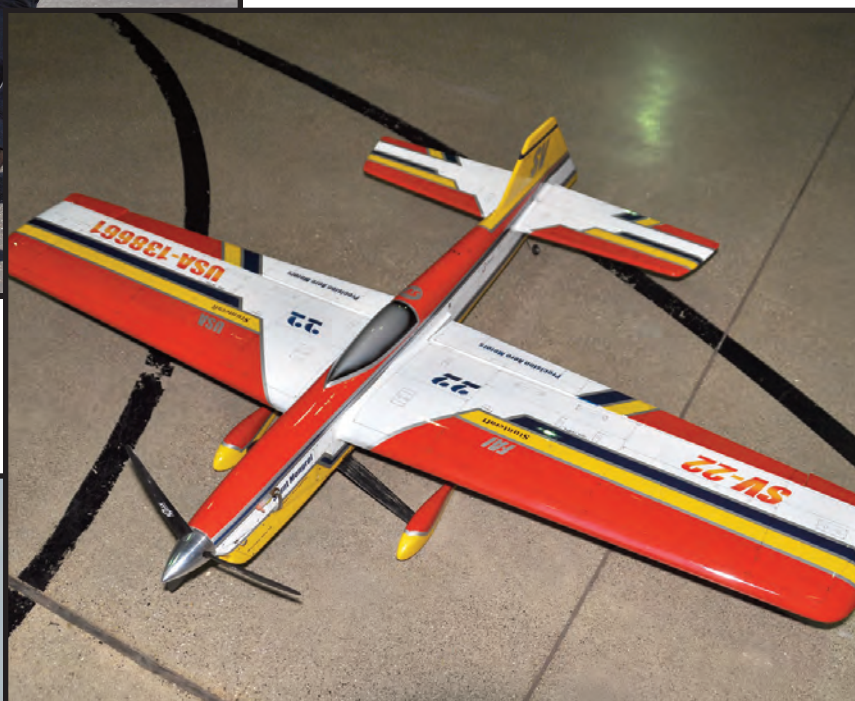
Above: The trim schemes on Bill Rich's planes are always colorful and original. This year's effort was just one more example of great craftsmanship and finishing technique for Bill. Power for this ship is a PA 65 with a Smith/Werwage carbon tuned pipe.
