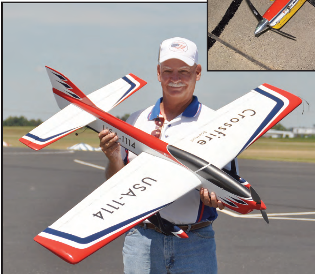
Above: The trim schemes on Bill Rich's planes are always colorful and original. This year's effort was just one more example of great craftsmanship and finishing technique for Bill. Power for this ship is a PA 65 with a Smith/Werwage carbon tuned pipe.
