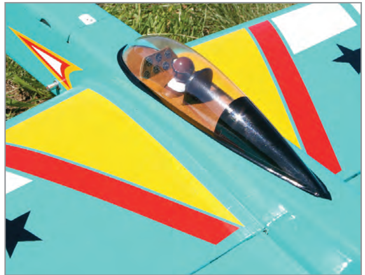
In this close-up photo of the cockpit area you can see the remote tuning pot that is used to adjust the RPM's. Note the DuBro Hatch Latch that secures the battery access hatch.
