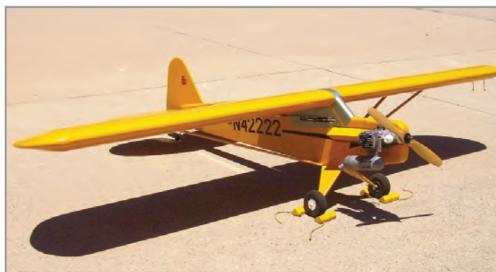
The Cub: Magnum .36XL power; N number same as Dale Gleason's Four Deuces full-size Cub; 465 sq. in. wing area; 22% tail; 40 ounces. I plan to have him fly it in the Warbird event at Baton Rouge.
