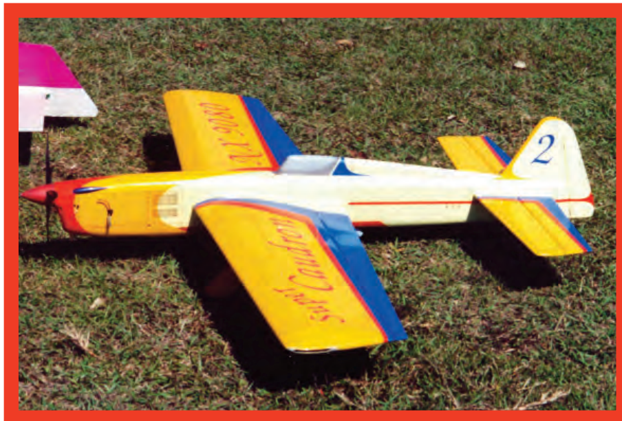
Super Caudron Number 2 again used the Magna series' wing and tail set. This model was originally built to accept an ST .60, but was later retrofitted with an OPS .40 and a tuned pipe.
