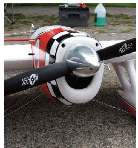
The nose of the Gee Bee looks pretty motivated! The “gun port” openings above the spinner are ports to reach fasteners to slide the upper part of the cowl forward to remove it. The big Stalker power plant is completely cowed in.
