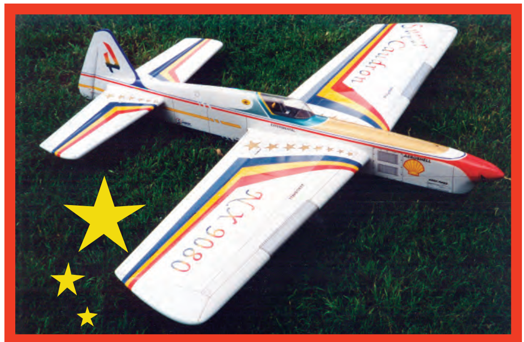
A total departure from the rest of the series of larger Super Caudrons, Number 4 was designed around Bob Hunt's 660-square-inch Saturn wing. This one was powered by a PA .51 fitted with a carbon tuned pipe.
