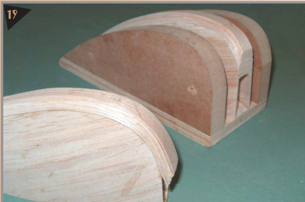
Fig. 17.) Glue them together and to the tip with polyurethane glue. It gives plenty of working time and is very easy to sand. Tape very securely making sure there are no gaps between strips. (See Fig 18.) Note that the strips don't go all the way around the leading edge.
