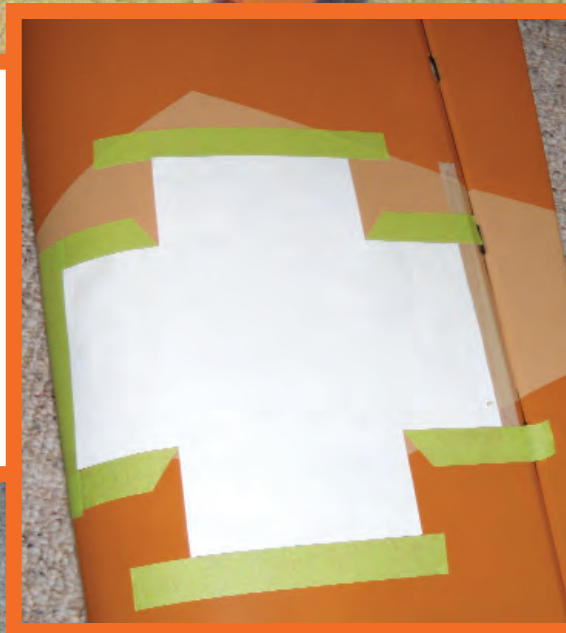
Above: The green tape is used to outline major areas for masking. In the case of my latest plane, I used it to outline the three major colors of my camouflage scheme: the two browns and the light blue.
