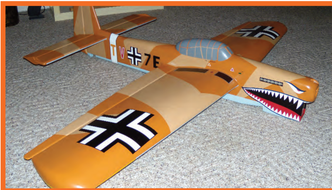
Left: Here is a picture of the completed masking and painting. What is missing is the ink lines, the decal for the rudder and the clear coats. This is to show you the many different possibilities that can be done with simple masking techniques. Apply these techniques to your particular paint scheme.
