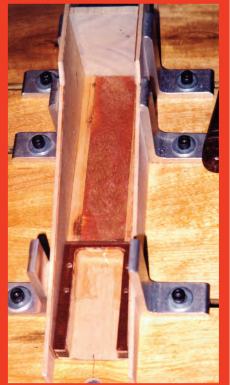
Here's the engine crutch assembly in the fuselage assembly fixture. Note the use of a 1/8-inch thick linen-based phenolic plate onto which the engine will sit (right).
