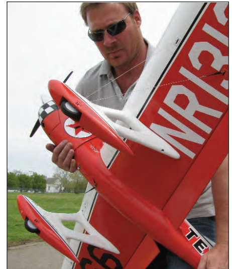
This view of the bottom of the Gee Bee shows the unique wheel pants Mike came up with. Also notice the external bracing wires that are on both top and bottom of wing. There is a miniature turnbuckle system to tension the wires. It's hard to see in the photos, but the wing also has dihedral.
