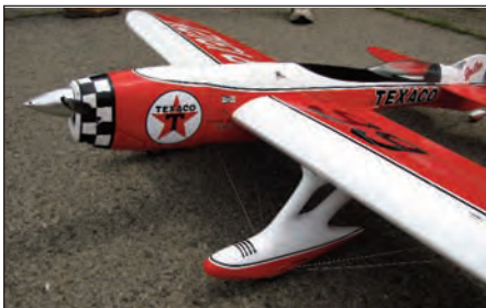
Mike's Gee Bee uses an interesting cowl system. The bottom opens conventionally, then the entire molded top and front can slide forward off the airplane, giving excellent access to engine and tank. The
