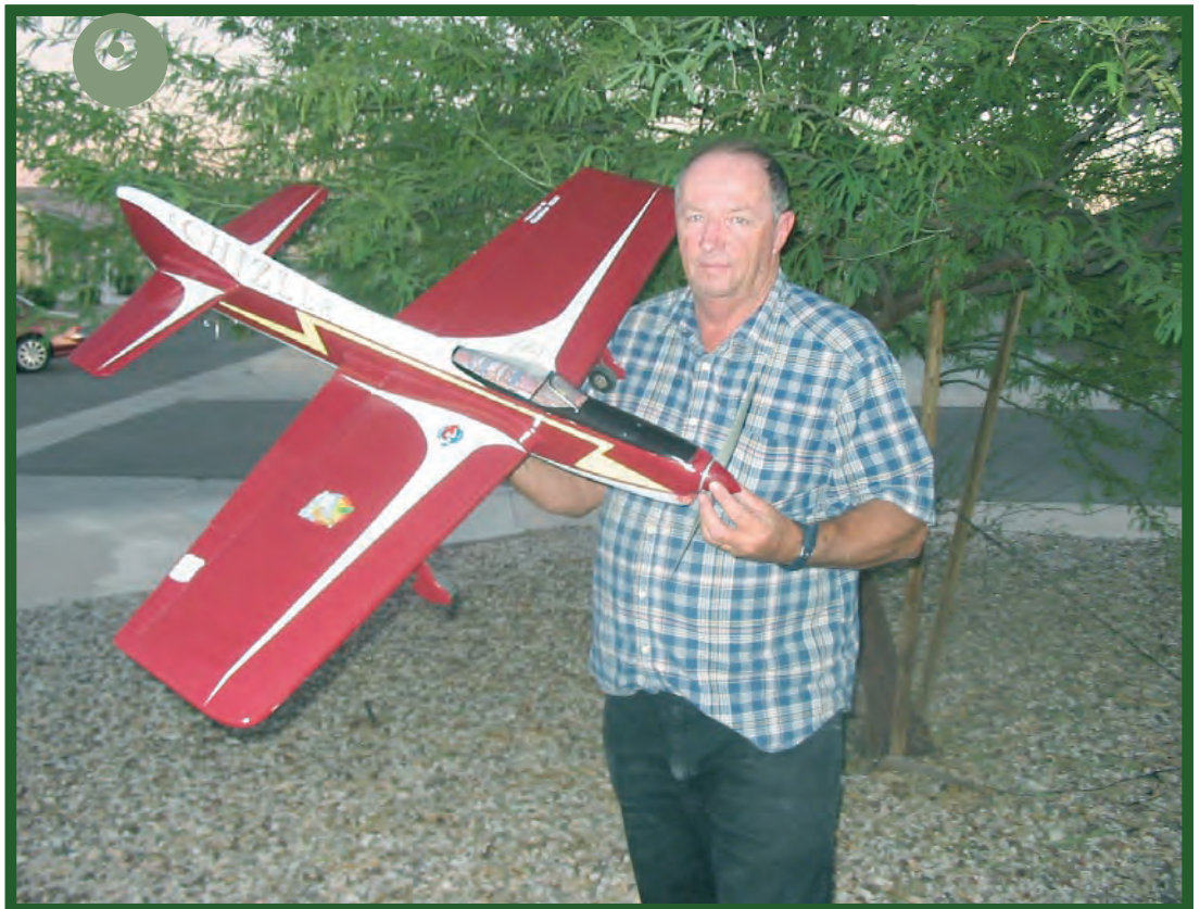
LeRoy Black with e-Chizler. If you look closely you can see the additional air scoop at the front of the anti-glare paint on the nose. You will need extra air inlets and outlets for electrics, and the air must also pass over the battery. The outlets are cleverly placed on the belly of the Chizler.
