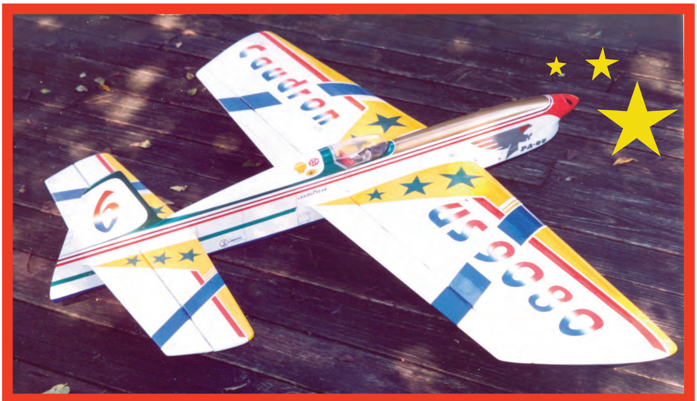
Super Caudron Number 6 flew originally with a PA .61, then with a PA .65 and then the cowl was modified to accept the mighty PA .75. Longer landing gear were also added to provide ground clearance for the larger-diameter prop.
