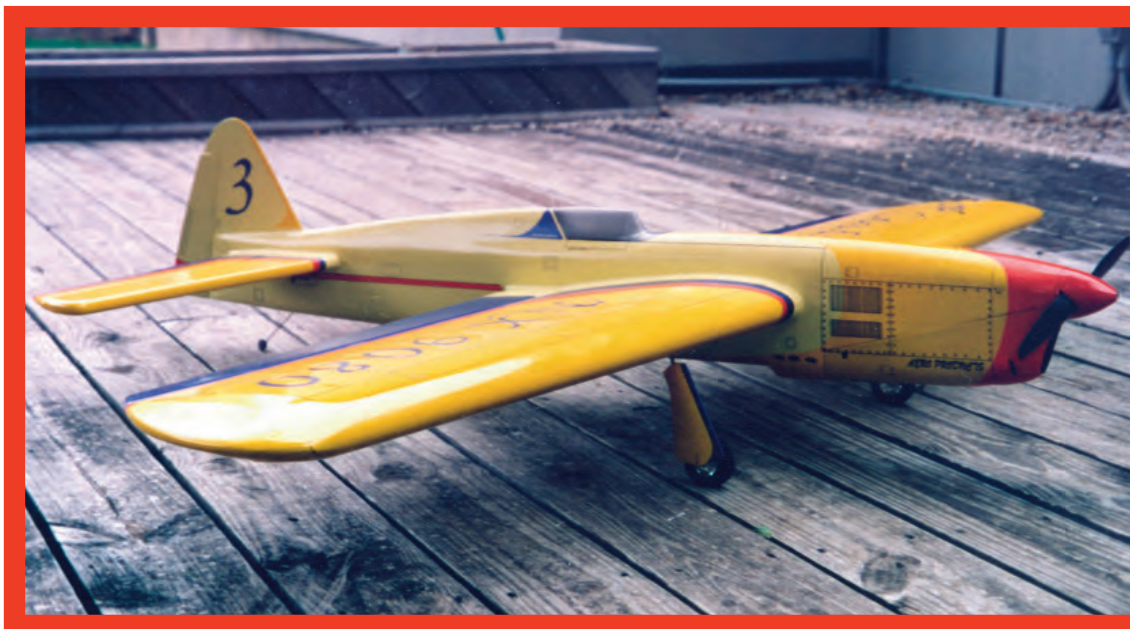
First of the series to be specifically designed to accept an OPS .40 and a tuned pipe, Super Caudron Number 3 utilized Bill Werwage's USA-1 airfoils, which were fairly thin.
