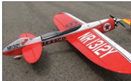
Another view of Mike's new Gee Bee. This model weighs 76 ounces, has 720-square inches of wing area, and is derived from the full-scale Cardinal in terms of moments, areas, and airfoils. Power is a Stalker .61 rear exhaust fitted with a Bolly 12 x 6 prop. Construction is built-up wing and fuselage, with both planked and molded skin. Covering is Super Coverite with painted finish.
