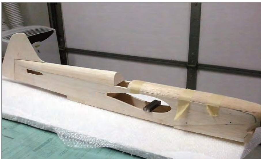
Side view of fuselage with built-up rudder, molded turtle deck, and hollowed front block, cowl etc.
