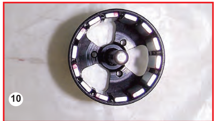
This photo (10) shows an inside view of the "can." The shaft is 5mm in diameter and is smoothly finished. There are 14 magnets. This is one place where I can see some money was saved. The magnets are not curved as in the Scorpion motors.
