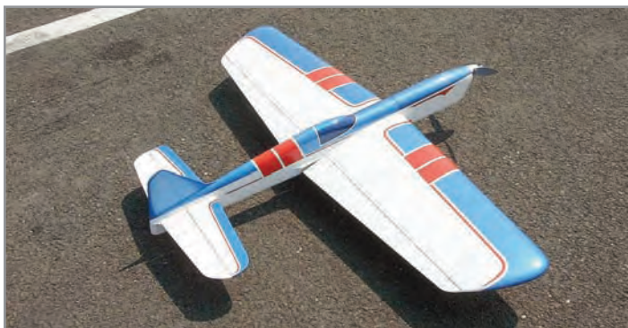
Above: Frank Imbriaco also built an electric powered Caprice. He powers this one with an E-Flite Power 15 motor and uses a Castle Creations Phoenix 45 ESC, a Will Hubin FM-9 timer, and a Hyperion 4S 2500 mAh battery. Below: Frank proudly poses with his excellently finished Caprice. He used the DuPont Chromabase paint system on this ship.
