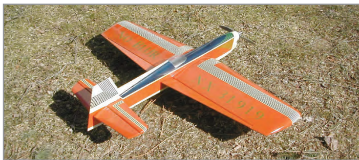
Tom Hampshire also built this Gieseke Nobler. It was built from an Ultra Hobby Products kit, and Tom fitted it with an E-Flite Power 15 motor, a Castle Creations Ice Lite 50, a Hubin FM-9 timer, and a Gens Ace 25C 2500 mAh battery.
