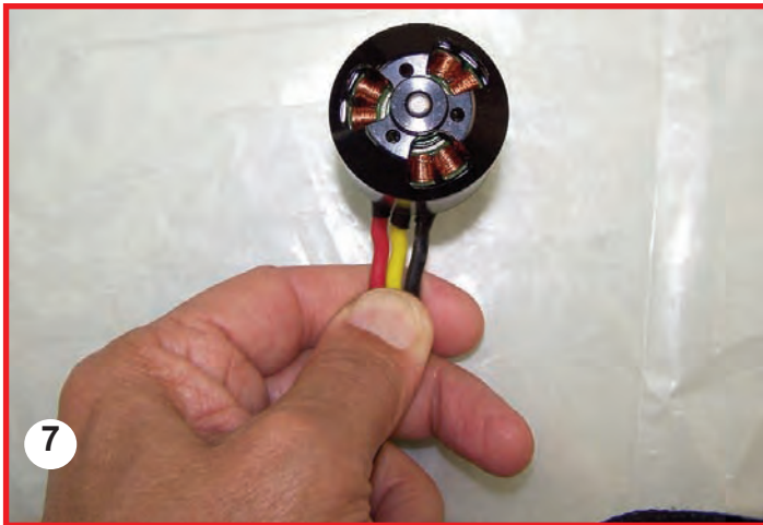
On to the back of the motor (7). It is evident that the effort was made to increase the size of the cooling holes. After removing the snap ring, I opened up the motor for examination.
