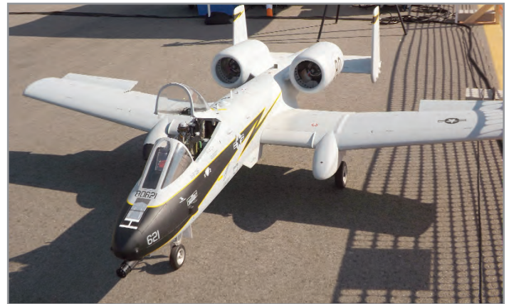
A scale model of the A-10 with twin turbine engines.
