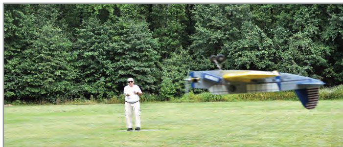
Above: Tom Hampshire prepares to hit the start button on his electric powered, original design, profile Vought Kingfisher, as Mike Kijesky holds. This model was designed around a Buccaneer 746 foam wing. Below: Tom's Kingfisher flies extremely well and is powered by a Scorpion SII-3026-890 v2 brushless motor. Other items in the power train include a Castle Creations Ice Lite 50 ESC, a Will Hubin FM-9 timer and a Hyperion 4s 4000 mAh battery. This model will be the subject of a future construction article in Stunt News .
