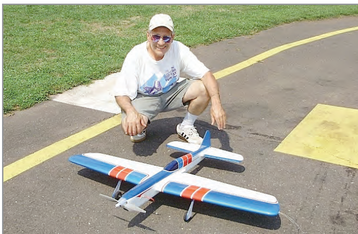
Above: Frank Imbriaco also built an electric powered Caprice. He powers this one with an E-Flite Power 15 motor and uses a Castle Creations Phoenix 45 ESC, a Will Hubin FM-9 timer, and a Hyperion 4S 2500 mAh battery. Below: Frank proudly poses with his excellently finished Caprice. He used the DuPont Chromabase paint system on this ship.
