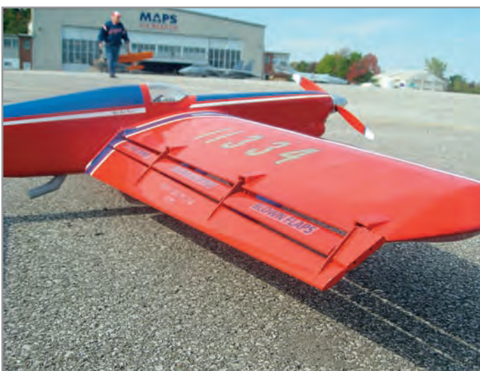
Wes Dick flew his original design Velvet in Expert and displayed his bi-directional, double-slotted flaps. Exotic!
