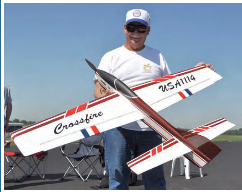
Here's Bob Hunt at the 2011 Nats with his new, electric powered, Crossfire Extreme. The model features a Masterflite foam wing that was cut and covered with the flaps integral to the airfoil. The flaps were then separated and framed with balsa. Photo by Gene Martine.
