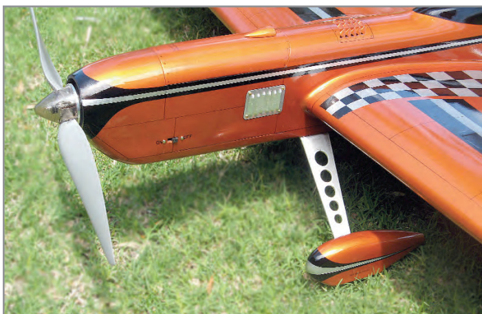
Above: There are lots of cooling louvers on John Callentine's new E-stunter.
