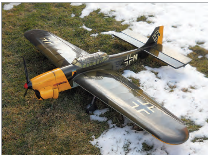
This angle reveals the wheel pants and the cowling details, as well as the carbon fiber 3-blade Bolly prop. Wieder photo.
