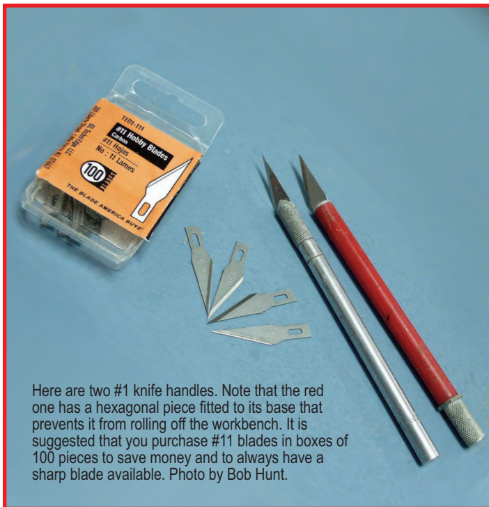
An even better option for most model cutting chores is a #11 scalpel blade. You can mount them in a surgical knife handle or break the tang and mount them in either a #1 knife handle or in an Uber Skiver handle—if you are lucky enough to have one or two! Hunt photo.
