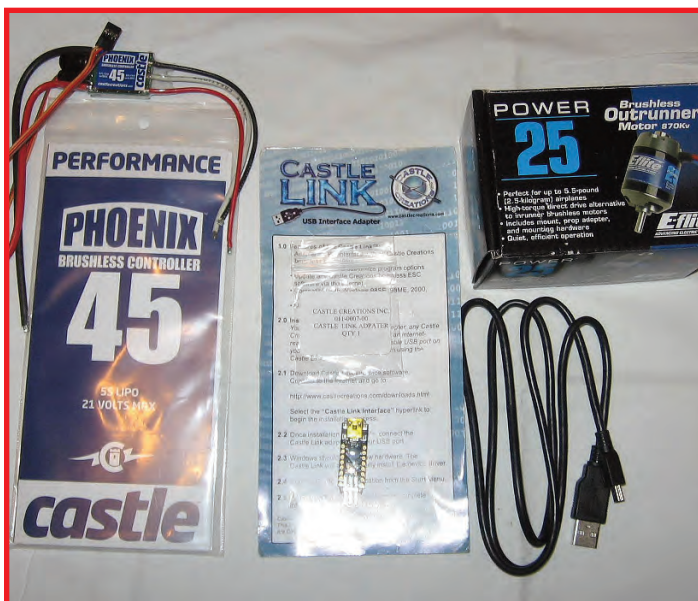
Photo 1: This shows the Phoenix 45, Castle Link, Mini USB cable, and the commonly used E-Flight Power 25 motor (870 KV version).
