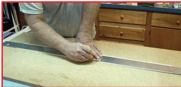
The ubiquitous #11 blade mounted in a #1 knife handle is the most common cutting instrument in modeling. Here that combination is being used to trim the edge of a piece of balsa in preparation to make up a set of foam wing skins. Watch the fingers! Photo by Robby Hunt.
