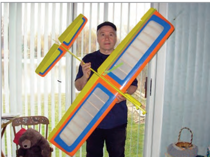
Dan Bregar's Pathfinder conversion will be powered by an Arrowind 2820/07 motor.
