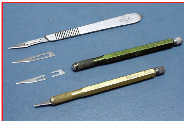
An even better option for most model cutting chores is a #11 scalpel blade. You can mount them in a surgical knife handle or break the tang and mount them in either a #1 knife handle or in an Uber Skiver handle—if you are lucky enough to have one or two! Hunt photo.
