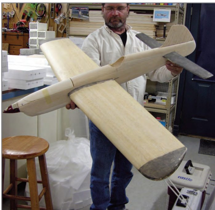
Alan Buck holds Bob Hunt's prototype Rounder in Bob's shop. This model features a "Reverse Composite" wing (a term made up by Bob...) and molded fuselage components.
