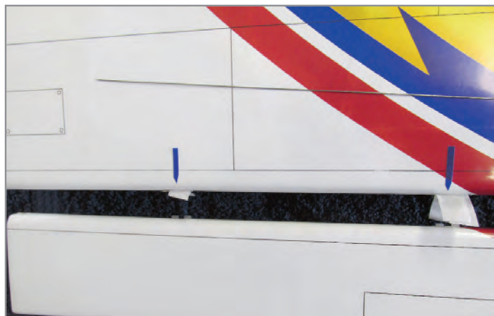
Thin CA has been applied. Be careful to use a small applicator and apply only a drop or two on the top and bottom. Be careful not to let the silkspan touch the finished surface. The silkspan at this point will be stiff and can be easily trimmed with a #11 blade. Haverly photo.
