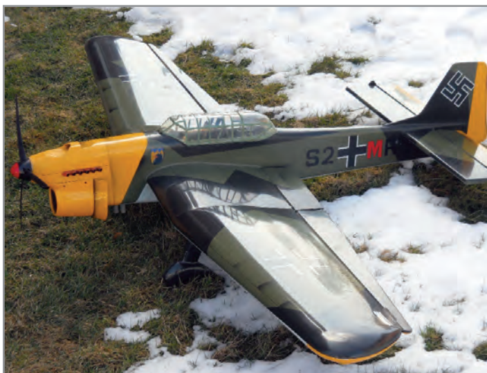
This Stuka has an inverted gull wing that was made from balsa covered foam. It has a wingspan of 67 inches. It is powered by a RoJett .90 engine. It nearly yanked Rich off of his feet! Weider photo.
