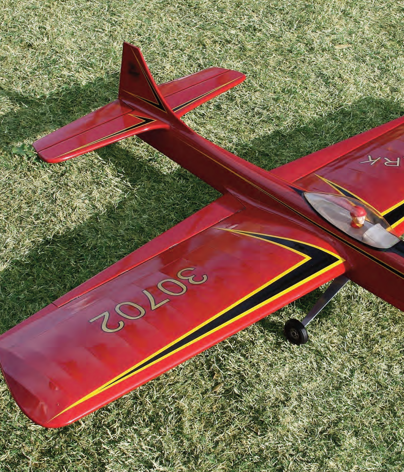
Paul Walker took a step into the past and brought this period-accurate Ed Southwick-designed Skylark to VSC and captured first place in Classic Stunt. It's powered by a McCoy .40 spinning a Top Flite 10 x 6 wooden prop!
