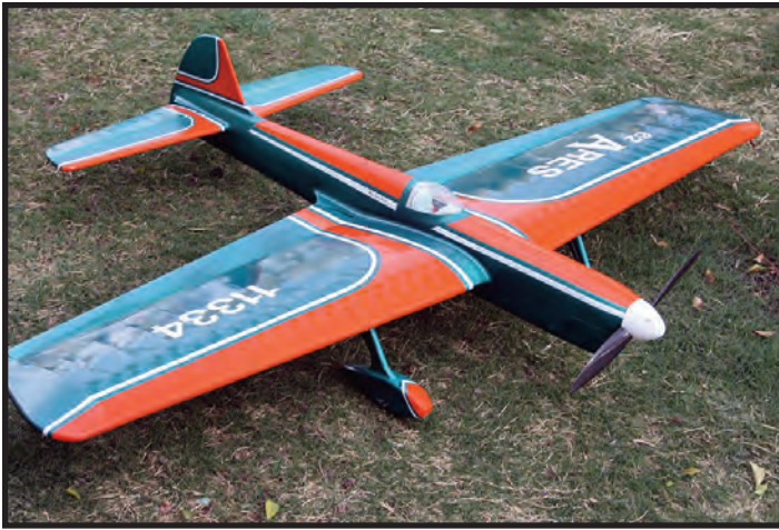
Wes Dick has been flying this Bill Werwage-designed '62 Ares for the past few years at VSC. It is powered by an Aero Tiger .26 engine and has a dope finish.
