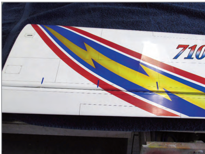
The offending hinges are identified with the blue marks. Photo by Mike Haverly.
