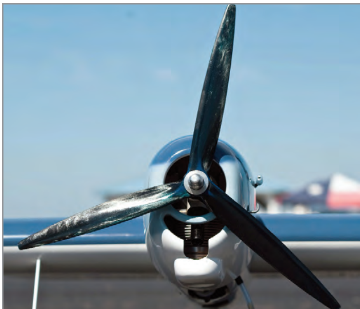
Business end of Kaz Minato's fantastic 2012 Nats front row F-6F-3 Hellcat. It features a piped PA-75 for power.
