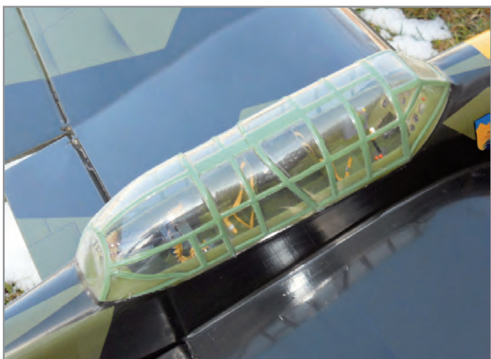
Here is the canopy on Rich's giant inverted gull-wing Stuka. Note the fantastic detailing in the cockpit. The canopy was molded for Rich by Dave Midgley. Wieder photo.
