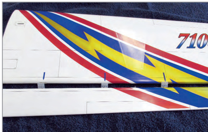
The new hinges are drilled out, deburred, lubed, and ready for installation. Haverly photo.
