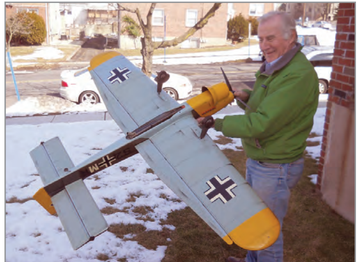
Rich gives us a look at the bottom of his straight wing Stuka, revealing the Smith/Werwage carbon fiber tuned pipe and the neat weathering detail that he applied. Wieder photo.
