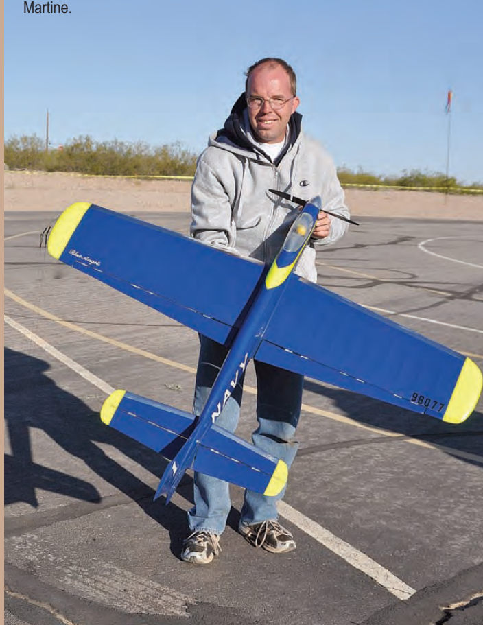
Steven McBride built this very clean replica of Larry Scarinzi's Blue Angel from a Brodak kit. It is powered by an ST 51 engine. Photo by Gene Martine.
