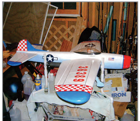
Bill Ballinger's T-Rex ARC with final trim and clear applied. A K&B .61 is the engine of choice. Bill Ballinger photo.
