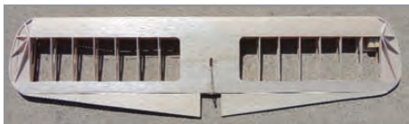
John Tate's Dolphin wing, done the "modern scratch-building" way: Draw your own plans in Autocad and then have the file sent to a laser cutter to produce a "kit" of your CAD file. Can't wait to see the finished model. John Tate photo.
