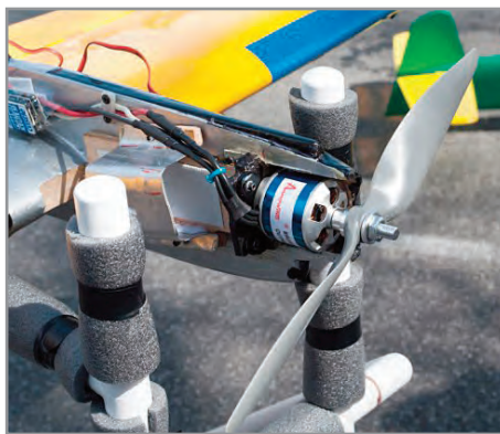
More and more planes in Central Virginia are turning up with electric motors in the front end. This is Jimmy Welch's P-40 ARC with an Arrowwind motor installed.
