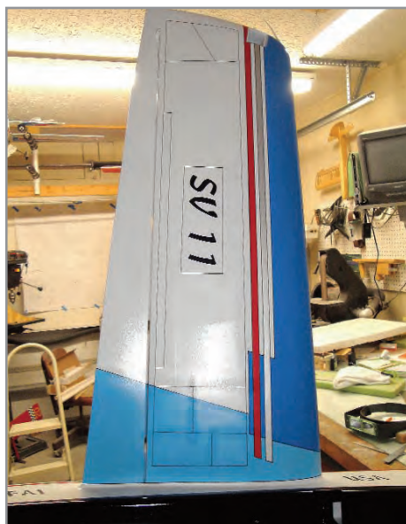
Bottom view of Martine's SV-11 with panel lines started. In the full-size picture you can see the little trails of clear he's shot over each panel line as he does them.
