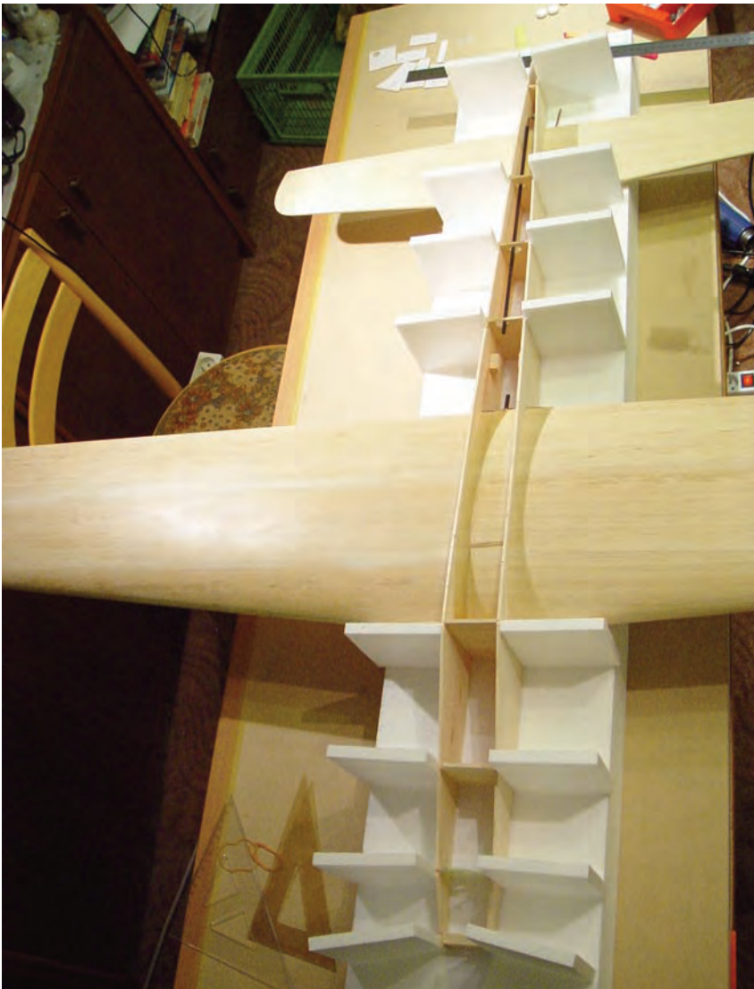
Igor prefers to build the fuselage for his models in a fixture and around the covered and assembled wing. He does not use a saddle cutout.
