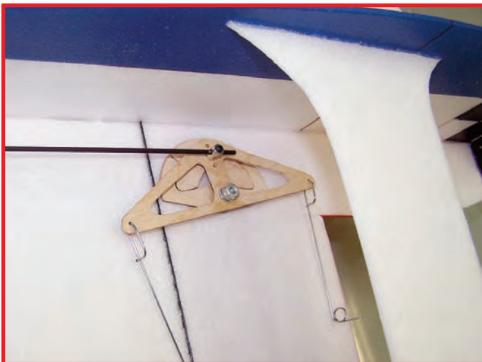
This is a close-up of the bellcrank and its mounting. I used .032 wire to form the leadouts. I also used a reduced throw on the pushrod location. It can be adjusted to any of the three holes for trimming.
