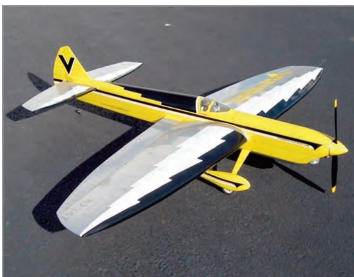
The Viper is fitted with removable Dural aluminum landing gear that is painted to match the model. The wheel pants are also removable to allow Joe to fly the ship easily off of grass fields. Note that the wheels are fairly wide. Joe feels that these wheels handle bumpy grass fields better than do thin wheels.
