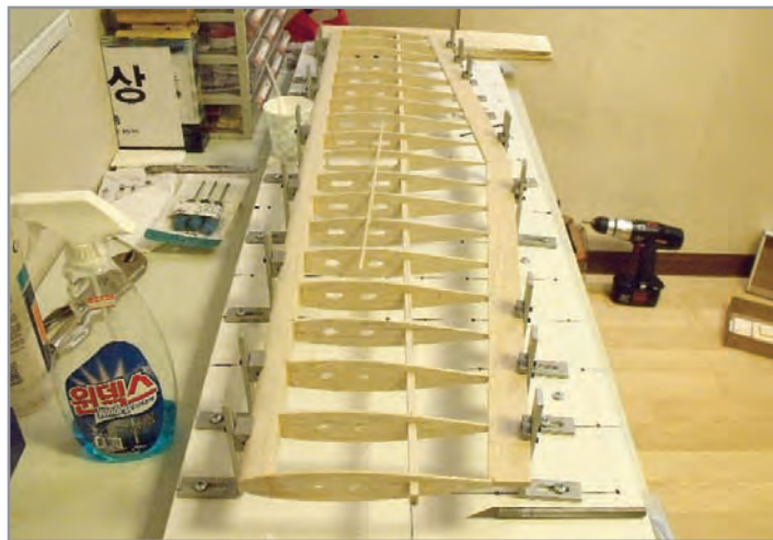
The Ringmaster wing is being framed up.
