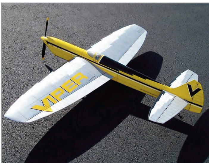
From this angle you can see that the Viper has a fairly long tail moment arm. Note how the wing and tail planforms virtually match.
