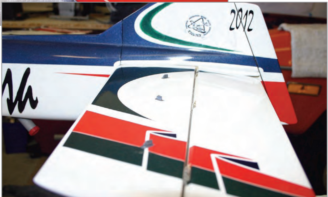
Right: Here are the Vortex generators on Dave Fitzgerald's Thunder Gazer tail.
