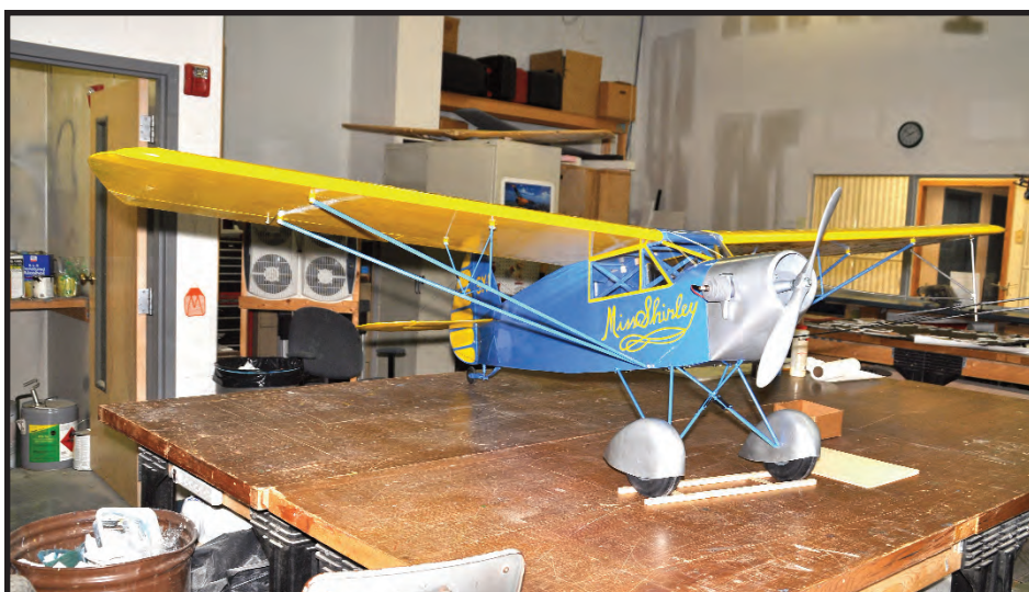
The size of the model was determined by the diameter of the propeller. The actual Miss Shirley was fitted with a 16-inch diameter, hand-carved propeller.
