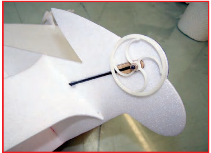
This is a 2-inch GWS wheel. The axle is solid 2mm carbon fiber rod.
