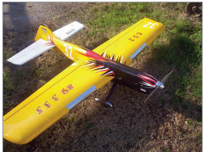
Jimmy Welch had been busy this past fall making a foam wing SV-22 for electric power. An E-Flite 32 motor pulls it with authority. John Tate photo.
