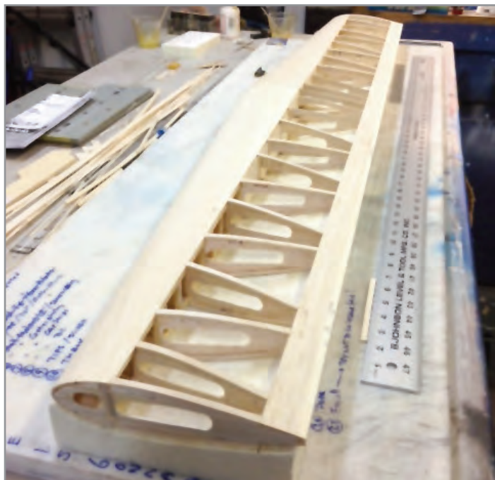
Here's my new Geo-Bolt wing setting in it's Lost-Foam fixtures.
