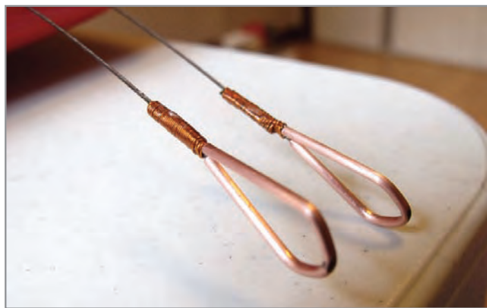
I tried copper tubing in place of thimbles.
