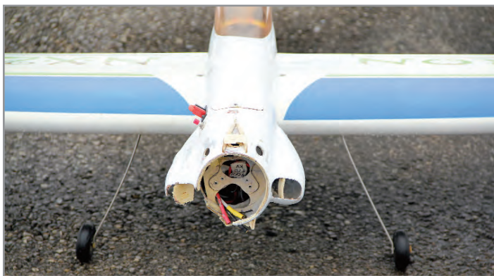
Jose's electric Shark seems to be missing something ...the motor! It seems that the motor mount came apart and the motor tried to do the pattern without the plane.
