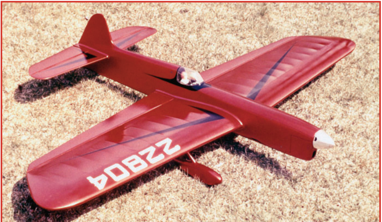
In 1966 Bob built and flew this “Simonized” Nobler. It featured a solid \frac{1}{4} inch thick balsa stab and elevator, wing mounted landing gear and more “swoopy” rounded wing tips. He used hollowed blocks instead of planking for the top and bottom of the fuselage. It was powered by an Anniversary version Fox .35 and weighed 45 ounces.
