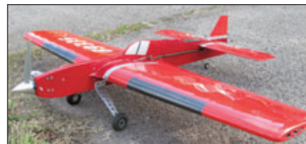
Another Welch project, this time an original design, using a TF Score wing, for the Saito 62. Another great-flying plane and one well suited to the winds found at the Virginia coast.
