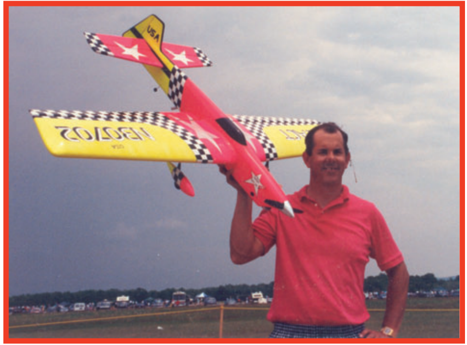
Paul Walker had a great year in 1992. He won the Nats and the World Championships that year flying his original-design Impact, fitted with an O.S. .40VF and a carbon fiber tuned pipe. Paul was the first to win the World Championships flying a piped model.
