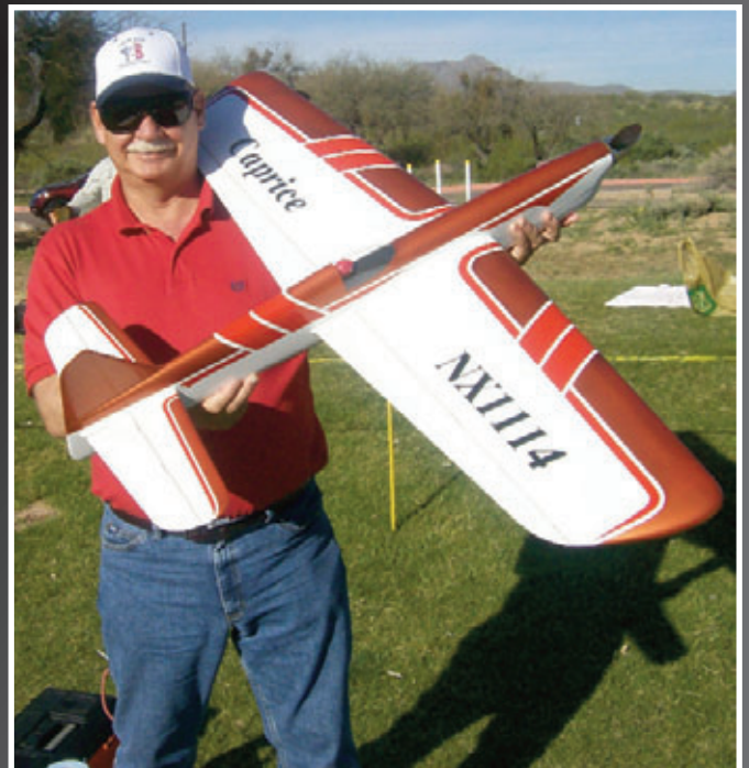
Here's Bob with his original-design, three-time Nats Classic Champion and three-time USC-winning Caprice. It features a foam core wing with triple internal coring. The original, built in 1967, also utilized a foam core wing.
