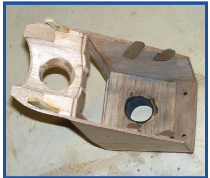
Here is a picture of the completed cowl with the carbon tube installed and sanded flush with the inside of the cowl.
