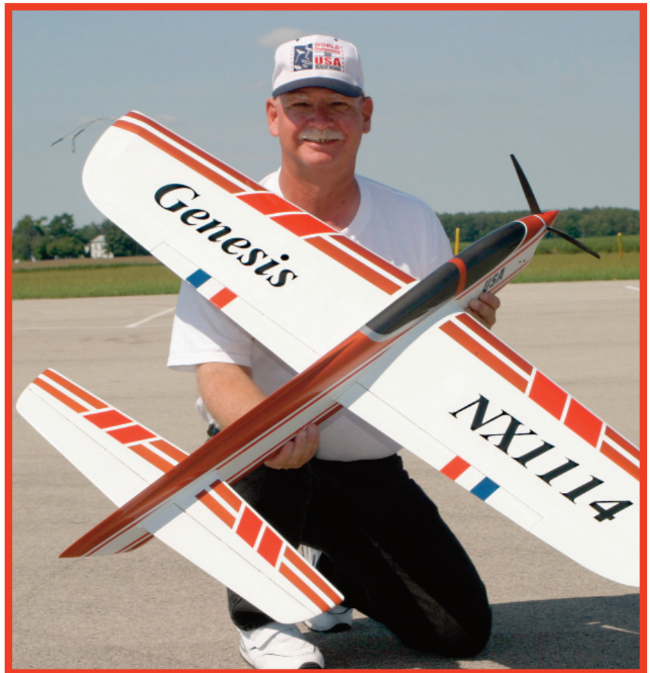
Bob Hunt retrofitted his Genesis Extreme with an electric power system and promptly captured a berth on the United States 2006 World F2B Team. He used an AXI 2826-10 motor, a Castle Creations Phoenix 45 ESC and a Thunder Power 4000mAh 4S2P Li-Poly battery. He believes electric power is the future of CL Stunt.
