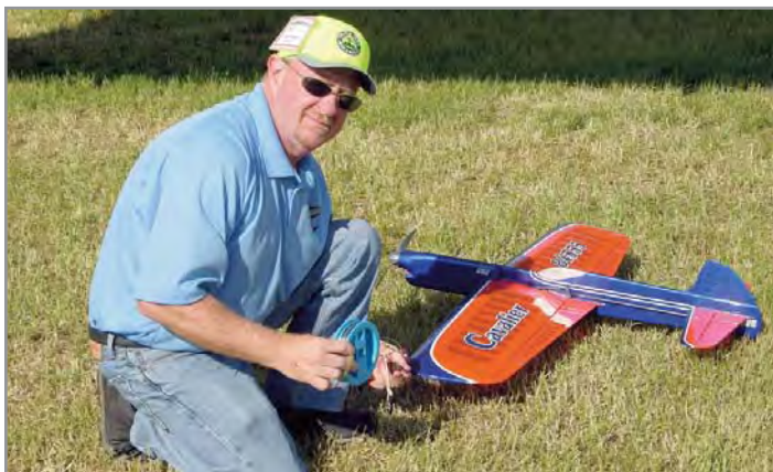
Bruce Jennings also brought a Tom Morris e-Cavalier to fly at the "Nall." It's powered by an E-Flite 25 motor with a Castle Creations Ice-Lite 50 ESC and uses a ThunderPower Pro Lite G8 2700 mAh 4S battery.
