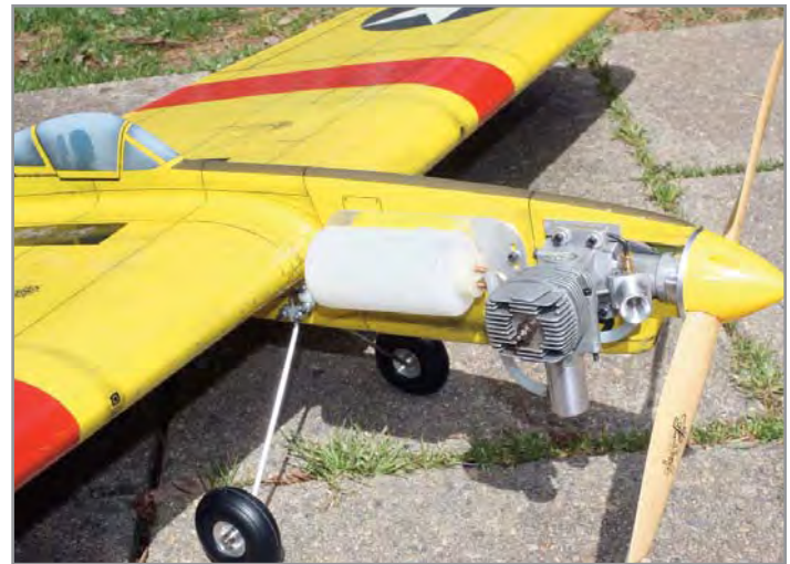
A view of the power unit. Tommy has a cleverly designed adjustable tank mount feeding fuel to the ST .51 crammed with "sekrit" modifications by John Tate.
