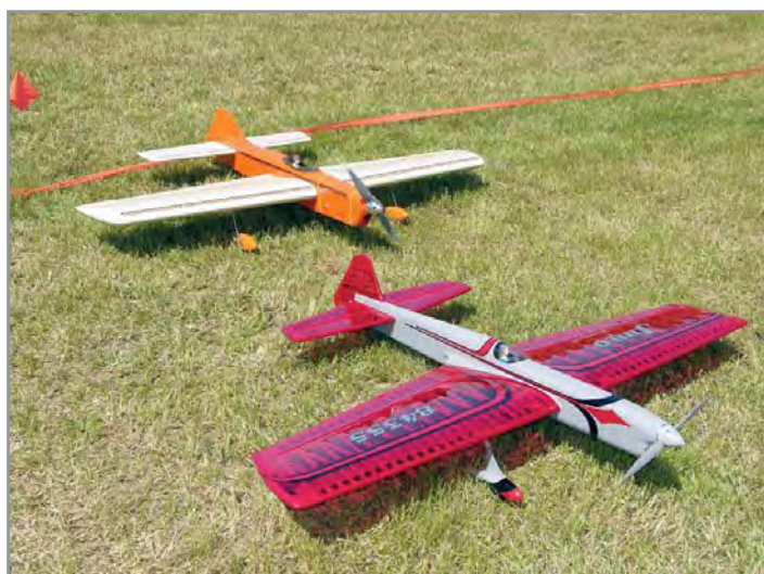
In the foreground in this photo is Bruce Jennings's stunningly beautiful, Bill Werwage-designed Juno. It is powered by an O.S. LA .46. The fuselage is finished with automotive paints and the wing and tail are covered with transparent MonoKote. Behind Bruce's plane is Fran Imbriaco's highly modified SV-11 ARC. Frank recovered the ship and painted the fuselage. He installed an E-Flite Power 32 motor and runs this combo on a 5-cell pack.
