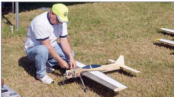
Bob Hunt prepares one of the "committee-built" Joe Nall Cadet trainers for a hop. These trainers were full-pattern capable and featured E-Flite Power 15 motors and Thunder Power 2700 mAh 4S batteries. Photo by Mark Weiss.
