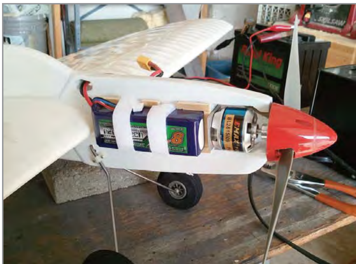
Chip Largent's Sig Banshee set up for e-power. The quiet power system will allow Chip to get back into CL flying right by his house.
