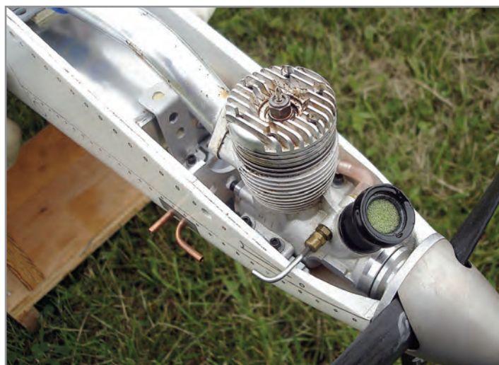
The Stuntquest features a very interesting and new engine and tank installation scheme. See the text for details. Polk photo.
