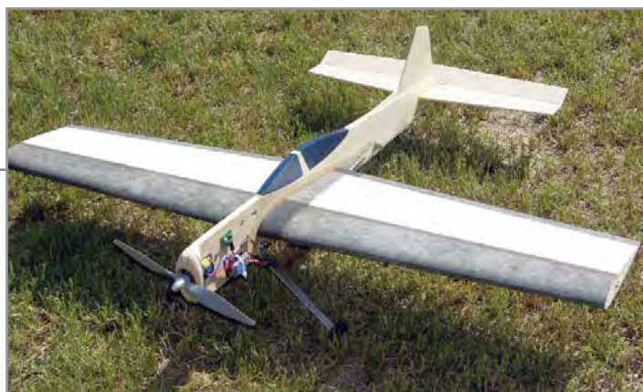
The Joe Nall Cadet features "Lost-Sheeting" wing construction with .2 ounce carbon mat applied directing on the foam in high stress areas using water-thinned Titebond glue. The ships were powered by E-Flite Power 15 motors, and they used Thunder Power Pro-Lite G8 2700 mAh 4S batteries. APC 11 x 5.5EP props were used, as were Will Hubin timers and Castle Creation ESCs. It was a true joint effort. Plans will soon be available for this ship, according to Bob Hunt.
