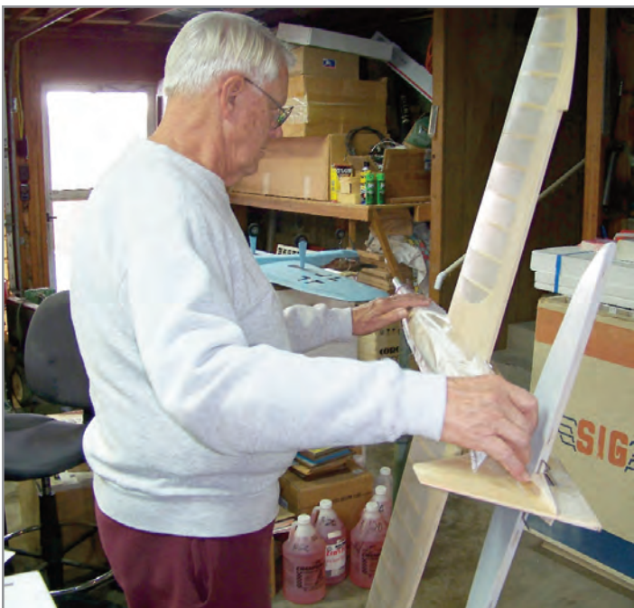
Here's Charlie Reeves with his new Ed Southwick Lark. He is applying light weight fiberglass cloth with an epoxy mixture. He covered the bottom in one evening, and then went to one side of the fuselage and rudder. Once that was cured, he was finishing up the last remaining side when this shot was taken.
