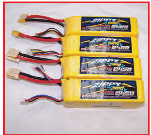
For power, the batteries chosen were Zippy Compact 5S 2450 mAh 35C-rated units.
