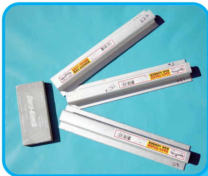
These are my most used blocks for sanding. As you can see, I keep different grits on each one and they are labeled so I can quickly choose the one I want. The smaller Black block is a "DuraBlock" hard foam sanding pad. It is very firm but has enough give not to cut flats onto rounded surfaces. I typically keep 120 on one side and 240 on the other.
