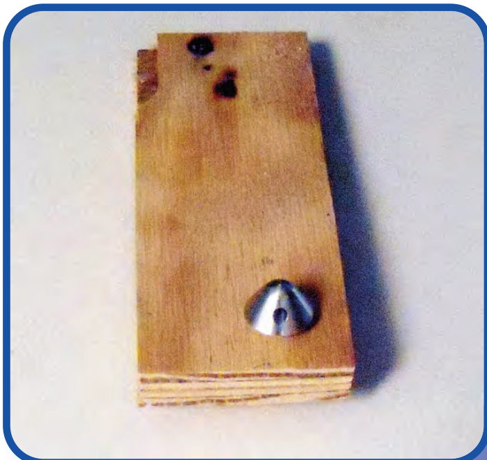
This is a picture of how I drilled a hole in a piece of wood to accept the nose section of the spinner.
