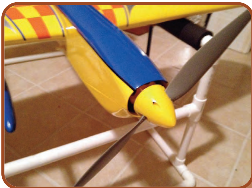
Jason's model uses the nose air inlet for cooling. Greer photo.
