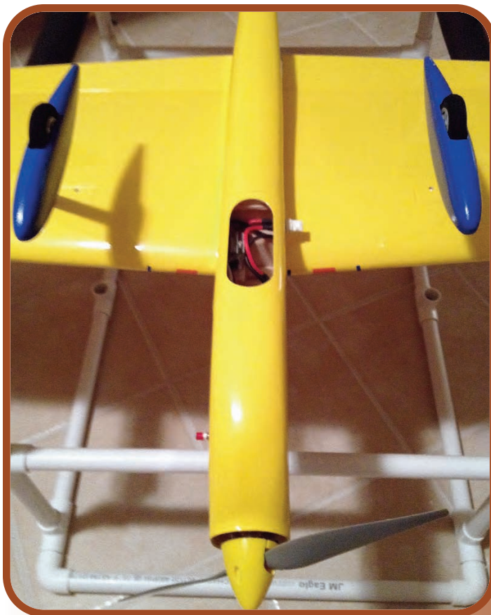
A bottom view of the GEO-XL that shows how clean the model is and the cooling air exit hole. Greer photo.
