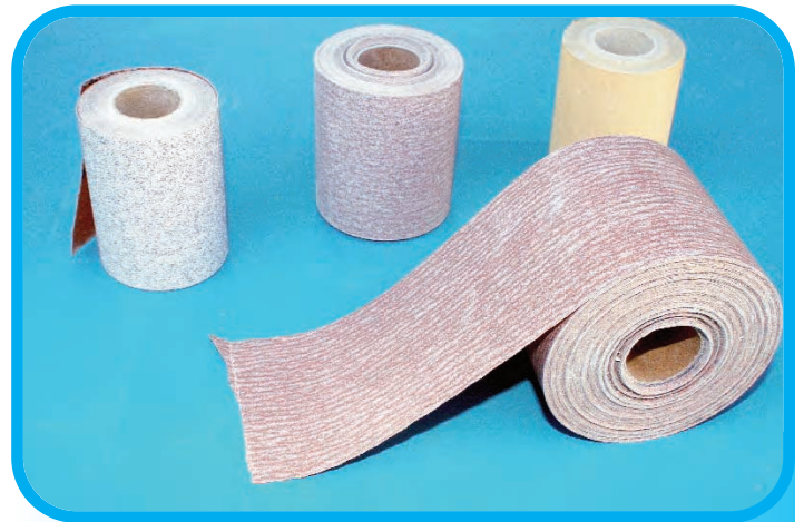
PSA 2½-inch sanding paper, these are the four grits I typically keep close at hand: 80#, 120#, 240# and 320. I also use 400# occasionally when dry sanding primer. This is the cat's pajamas for sanding, convenient, good quality, and easily affixed to virtually anything to use for a shaping block.
