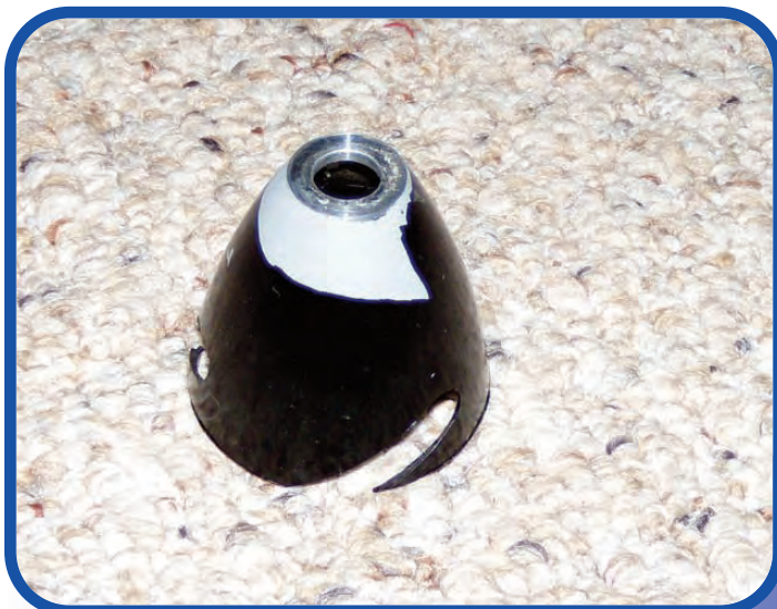
Here is a shot of what happens when the paint does not stick and starts to chip. Not a very pretty sight.
