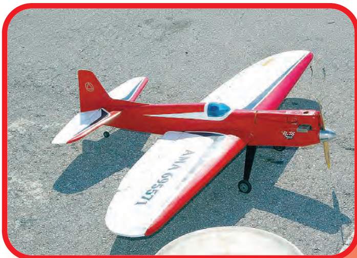
The Upright Thunderbird. It gets its name from the upright engine installation. There is also one with an inverted engine and they both fly very well.
