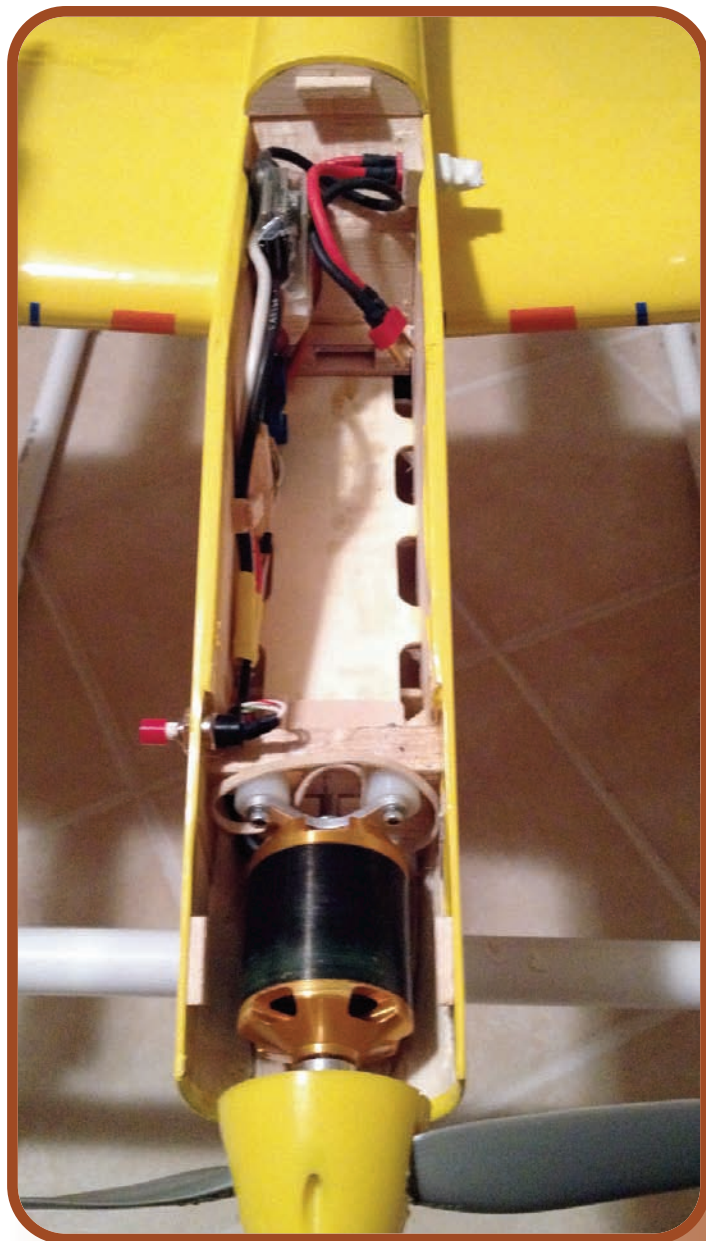
Bottom view with the cowl removed. Notice the rubber band that Jason uses to hold down the front of the cowl. Also notice how Jason has positioned the battery to the outboard side of the fuselage. Greer photo.
