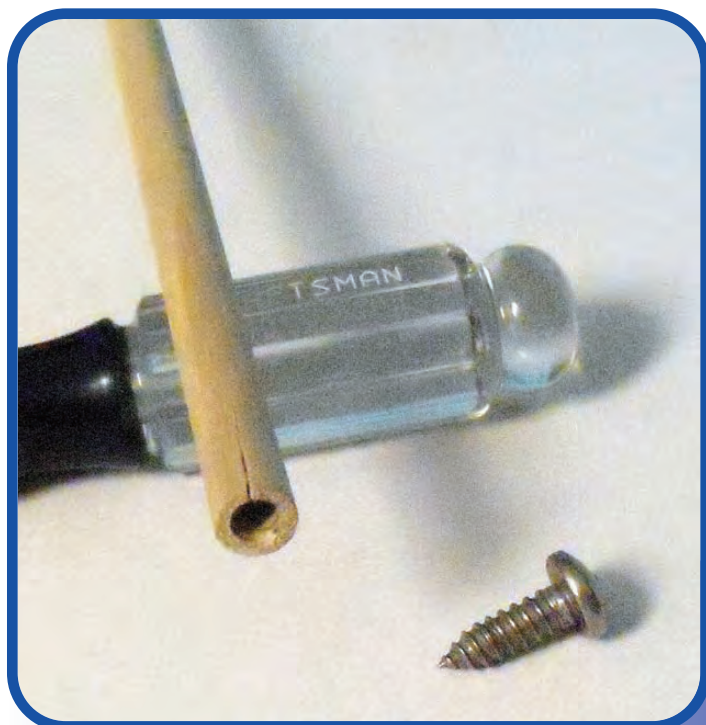
Here is a picture of the dowel that I used with the hole drilled in the end. Note the large head screw. You can use a washer under this to hold the spinner backplate.
