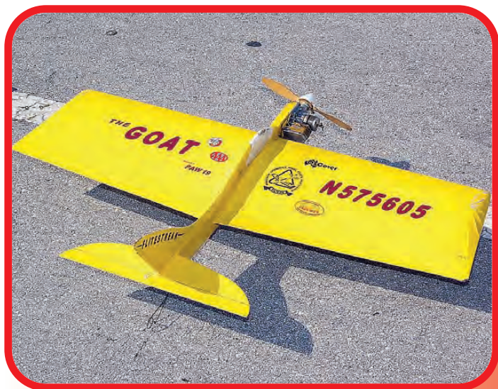
This is a Flightstreak, a good plane to get started with. Just like a Ringmaster it is small and flapless. Either of these planes will work in Basic and Beginner.
