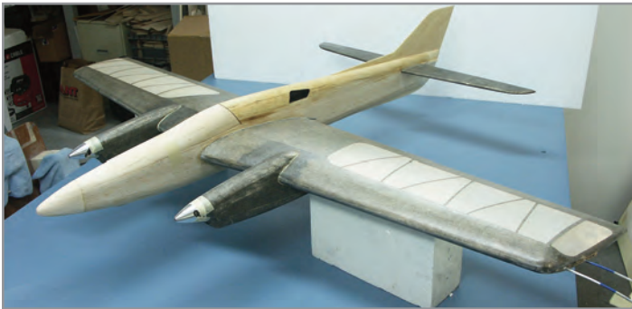
Second Wind is the name Bob Hunt chose for his new electric twin-motor stunter. It will be powered by two E-Flite Power 10 motors and one Hyperion 4S 4000 mAh battery. Photo by Bob Hunt.
