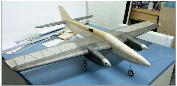
With the gear down there is plenty of clearance for up to 11-inch diameter props. Lots of disk area! Hunt photo.
