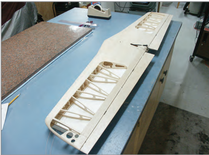
Here the wing is complete. Note that the center section sheeting runs out past the nacelles. This allows for a more rigid mount area for the nacelles and more center section strength. Hunt photo.
