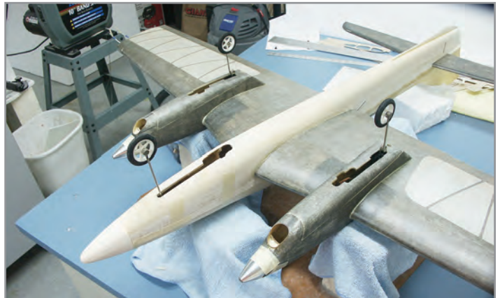
Twins with nacelles make retract installation and operation very easy to accomplish. Hunt photo.
