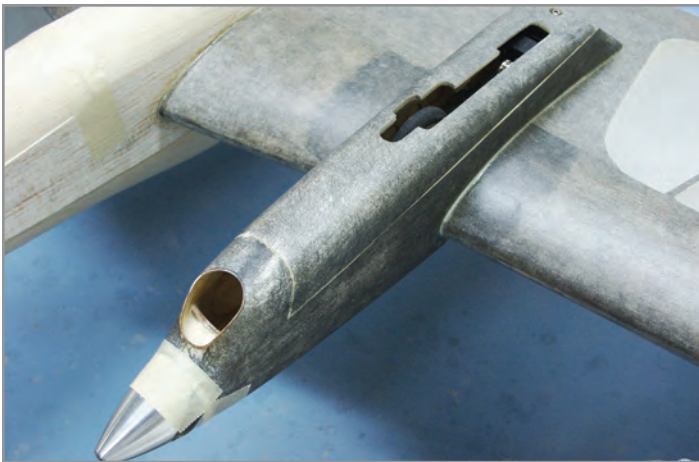
Here's a shot of the underside of one of the nacelles. Note that the retractable landing gear rotates forward through a clearance hole in the nacelle's hatch cover. Hunt photo.
