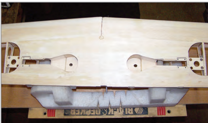
This bottom view of the wing shows the wheel wells and the main landing gear mounts. Hudak photo.
