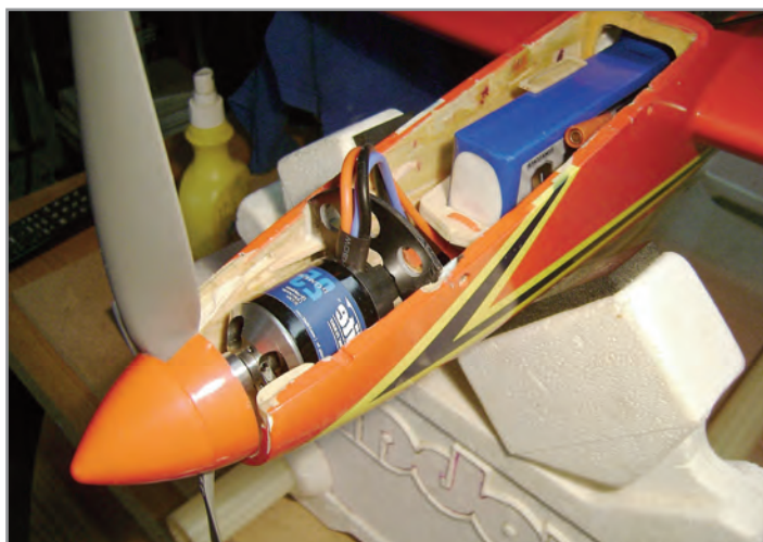
An E-Flite Power 25 was Dave's choice of motor for the Skylark. All the components fit nicely and the installation looks "stock." Note the reverse-pitch, or "pusher," APC prop. Heinzman photo.
