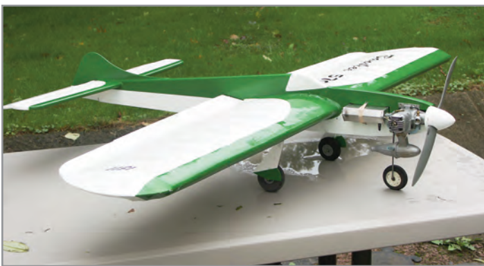
Perry's Banshee was modified to include tricycle landing gear.
