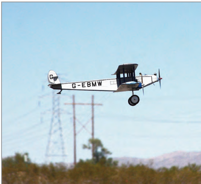
Lou Wolgast's 1/2A Multi Engine Scale model features two wings, three throttled motors, two rudders, and miles of rigging.
