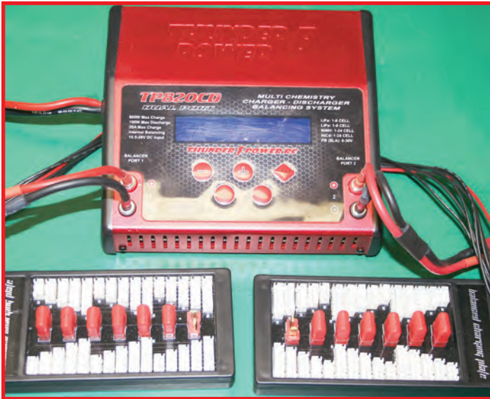
Thunder Power 820CD charger: This dual charger has 20 amps and 400 watts available out of each port. It is updateable and has good support from Thunder Power. Photo by Ron Heckler.
