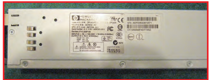
This is a typical server power supply. This one has yet to be repurposed for powering chargers. This might be the most popular one used and is readily available. It has an available output of 12 volts, 47 amps, and 575 watts.
