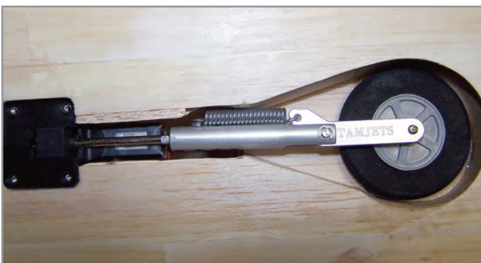
In this photo the landing gear strut is neatly nestled in its well. A very ambitious project! Hudak photo.
