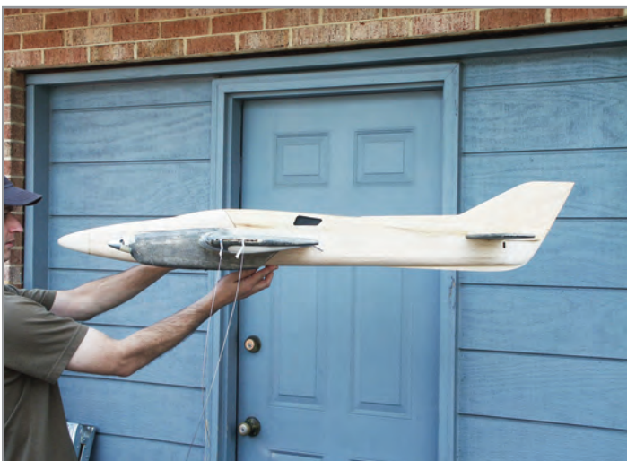
And here's a side view of Bob's twin. Note the air outlet vent in the fuselage side and the ventral fin. Bob hopes to fly this one at the upcoming Nats. Hunt photo.
