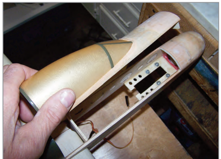
gear retract mount and the neatly painted canopy that is part of the removable top hatch. Hudak photo.
