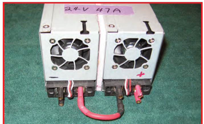
This shows two of the DPS600pb, set up and repurposed into a powerful 24 volt, 47 amp, 1150 watt power supply.
