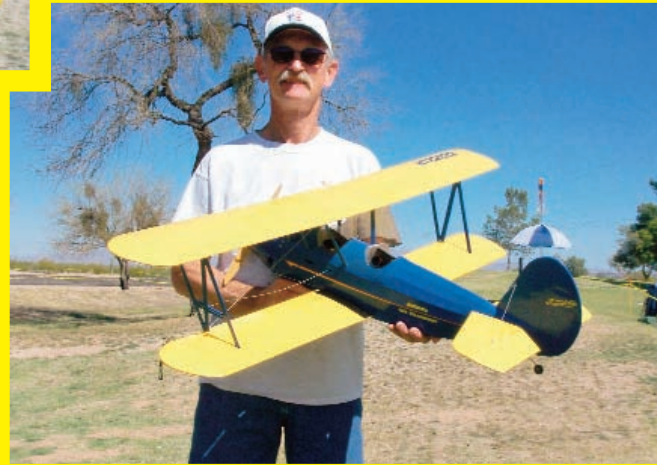
Below: John Callentine stuffed a few more ponies in the nose of his Jim Hunt designed Travel Air biplane. It now sports an LA .46. An outstanding piece of craftsmanship!
