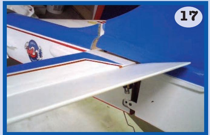
Slide in the vertical stab.
