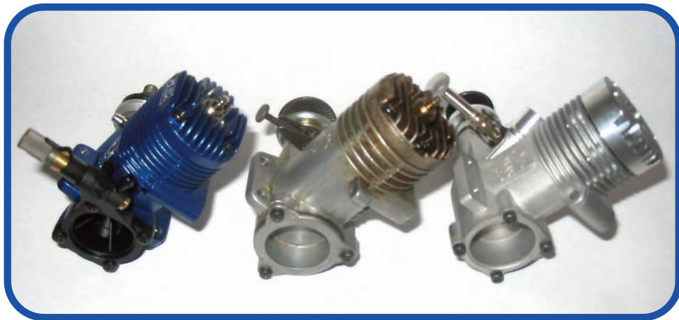
The backplates are the key feature for this shot. You can't help but notice the LA has a remote built-in needle valve, the other two have the conventional backplates, and the just-behind-the-prop arrangement for needle valves. Many .25 LA fliers opt for the metal backplate and either the standard needle valve, or the remote needle valve like the .40-.46 needle valve noted in the text.
