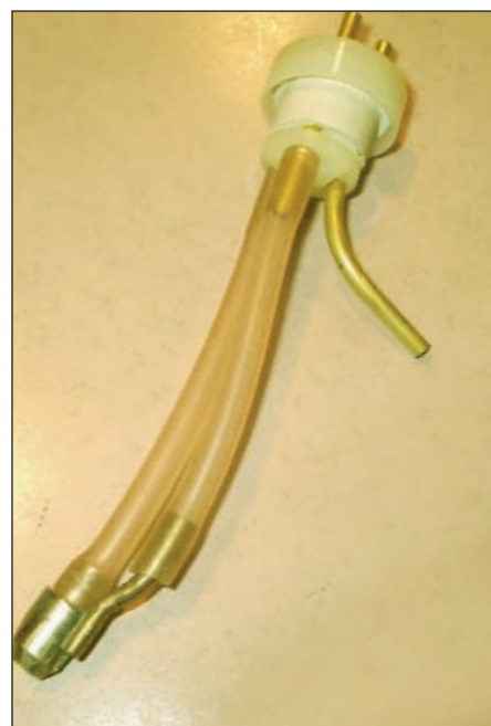
This is a Tom Morris plastic fuel tank unflow setup. It works well and is simple.
