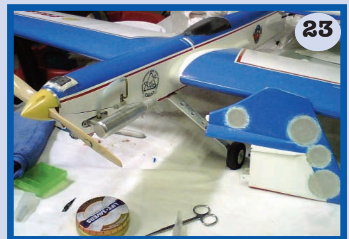
Lightening up the vertical stab saved only 2 grams. Still, it was worth it!
