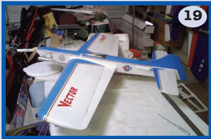
When it's all together, tape around wing joints and you're ready to fly. (What a messy garage workshop, I just realized!)
