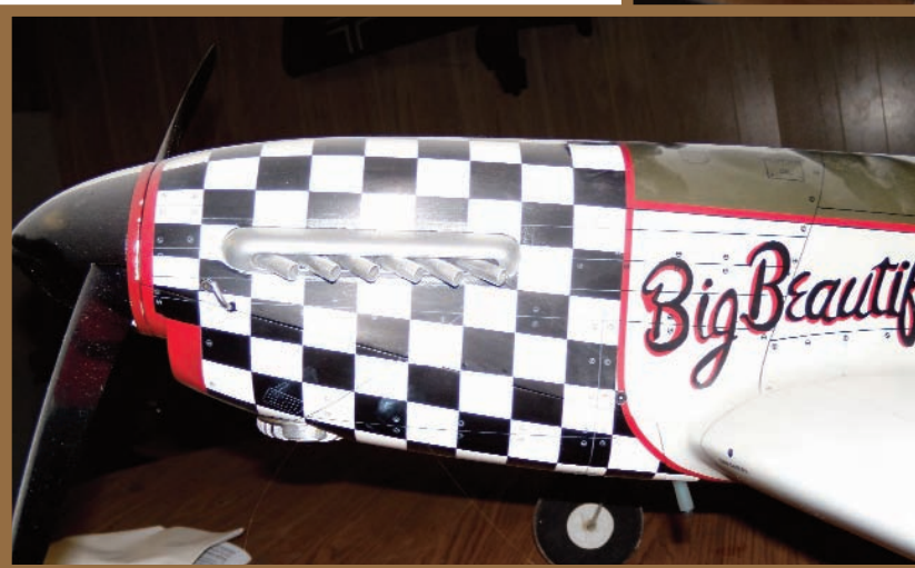
Here is a picture of the exhaust stacks on my 2002 plane. The full-scale Stuka has a fairing of some kind over the front of the first exhaust pipe with an opening in the front of the fairing. I just put the screw hole where the front hole of the fairing would be. This helps to "hide" the bolt hole even though it is in plain sight.
