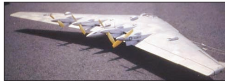
XB-35 ready for test flight. Four McCoy .35 engines buried in the wing driving props through extension shafts.
