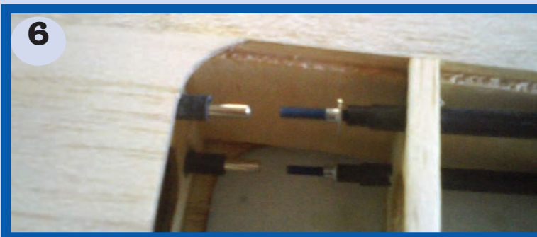
This photo shows the wing tubes screwed on to the outboard wing. A 2-inch-long 4-40 bolt is inserted into one of the \frac{3}{16} -inch-I.D. carbon tubes and the blind nut is glued to the bolt so that it won't fall out from the right side of the carbon tube. What prevents the bolt from falling on the left side? A \frac{1}{2} -inch-long, \frac{3}{16} -inch-O.D carbon tube is glued into the \frac{3}{16} -inch-I.D. guide tube. They need to be glued properly since all forces are transferred to this area when both wings are tied together.
