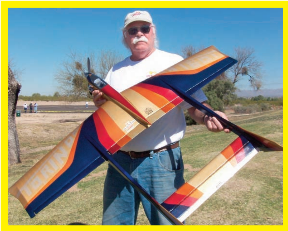
John Miller likes twins—usually twin-engine models, but this time a twin-boom model! He built this Jack Sheeks designed Torino for Classic Stunt. It's powered by a Fox .35.
