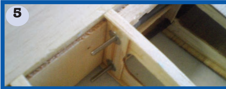
This photo shows the wing tubes screwed onto the inboard wing. Make sure that reinforcement is done properly around this area.
