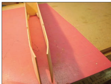
This photo shows Dave's Jaguar fuselage rear end detail. He used 1/64-inch plywood to shape the fuselage sides to give more room for the controls. Heinzman photo.
