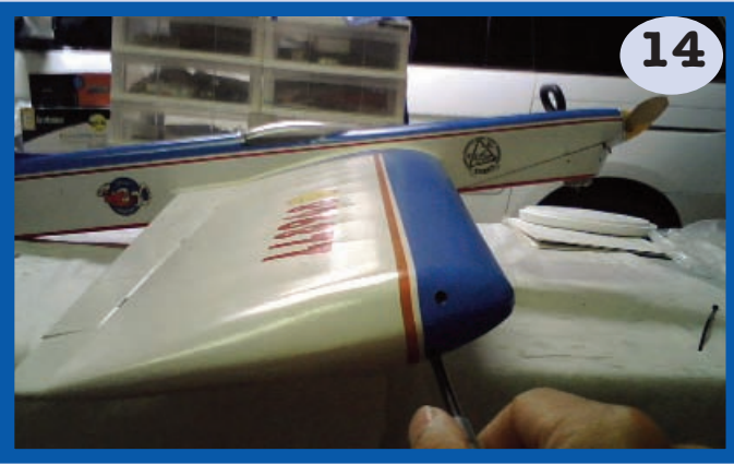
Screw in the holding bolts to the wing tubes through the outboard wing tip. The long screw driver is made of \frac{3}{16} -inch-O.D. carbon-fiber rod with a sawn-off socket-head ball driver glued to the tip.
