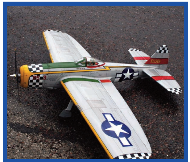
Bob built three Billy Werwage P-47 Thunderbolts. This is the third one and it is powered by a PA .75 with a pipe. Note the intricate panel detailing and the abundance of fine paint trim.
