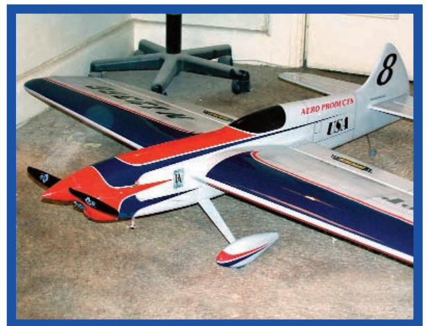
Here's Bob's original design Viper 8. It weighs 52 1/2 ounces and is powered by a PA.65 with a pipe. Bob likes lightweight stunt models and his building techniques will help others to achieve lighter models as well.
