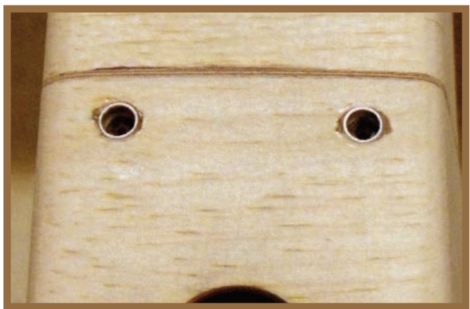
This is how the end result should look. The tubes have been carefully ground off and finished with a sanding block and 180-grit sandpaper. You may have to take the end of a dull number 11 blade and clean out the inside of the hole. Notice I said dull blade. If it is not dull before, it will be after you clean out the hole. This is one of the few cases where a dull blade is actually preferable to a sharp one.
