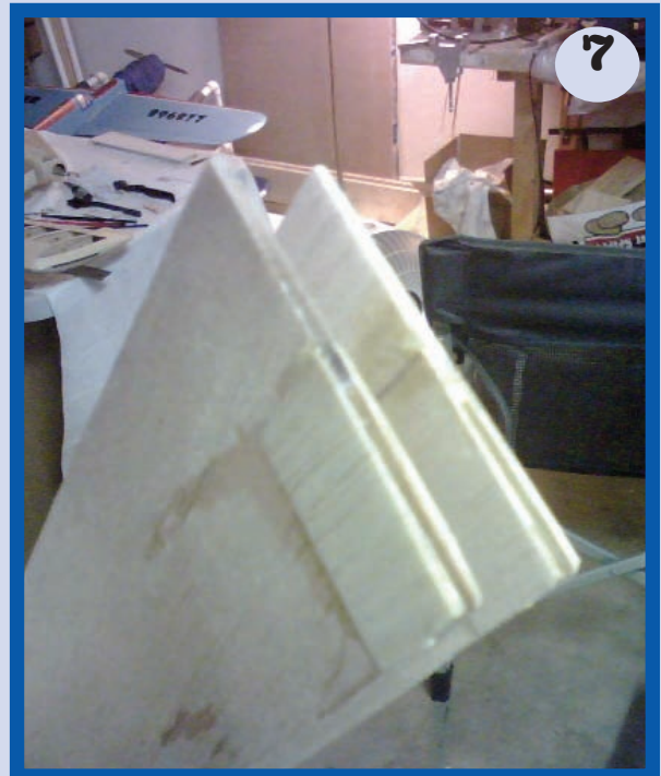
A "Lucky Box" is used so that it is possible to slide the control horn wire into the end of the flap. The control horn wire needs to snugly slide into the Lucky Box to avoid the sloppy control. The Lucky Box is constructed from plywood.
