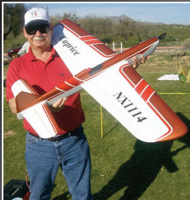
Here's Bob with his original-design, three-time Nats Classic Champion and three-time USC-winning Caprice. It features a foam core wing with triple internal coring. The original, built in 1967, also utilized a foam core wing.
