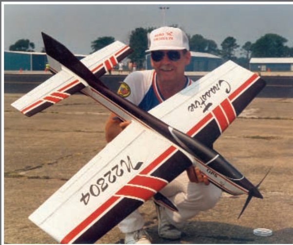
Bob Hunt's Crossfire featured a foam wing with integral foam flaps and a foam stabilizer and elevator. It also featured wing-mounted landing gear installed using Bob's innovative foam wing landing gear system.
