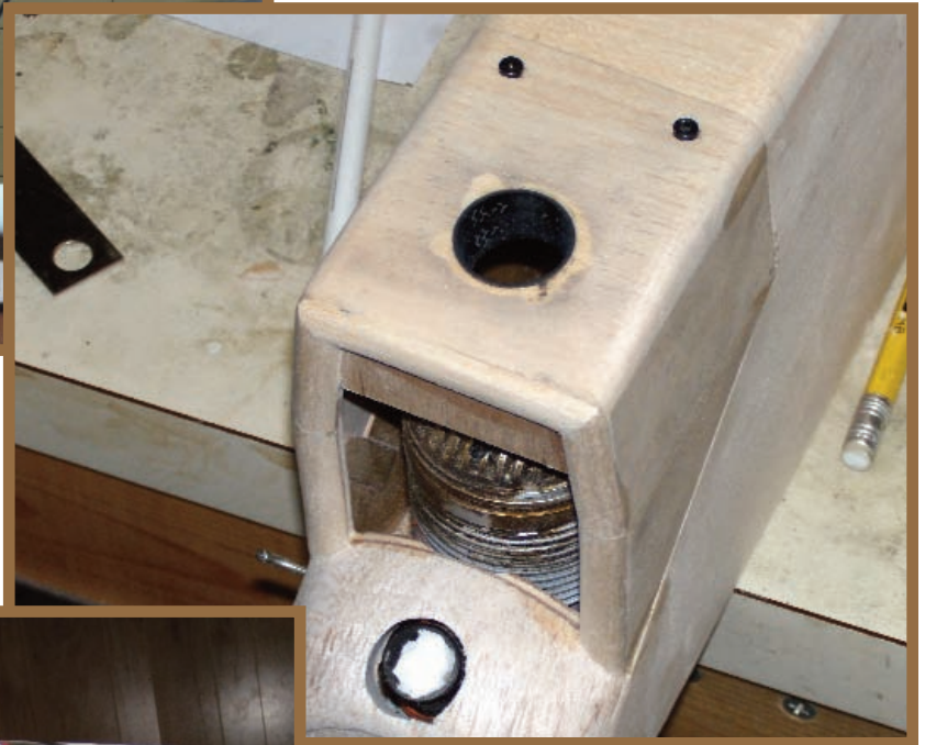
Above: Here is a shot of my cowl with the bolts snug enough against the balsa wood to hold the cowl in place but not so tight as to crush the balsa. I then drew a line around the bolt heads so I could use this as a locator for the outside diameter of the aluminum tubing.
