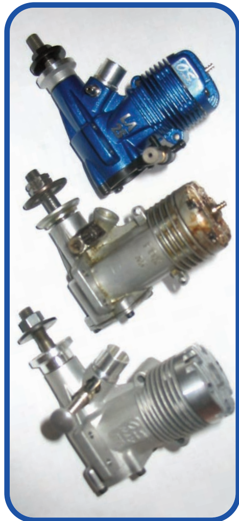
The three engines again, this time with a better view of the venturi and mounting lugs. The .25s do exactly interchange, and depending on your skills at finessing an engine they can be put into place with the Fox as well. Best bet is to re-measure and use two of the existing Fox mount holes with two new .25 holes.
