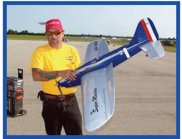
One of Bob's most unusual projects was his Supermarine S6B which was built around Billy Werwage's Thunderbolt "numbers." It is powered by a PA 65 that is fitted with a muffler. It weighs a svelte 58 ounces!
