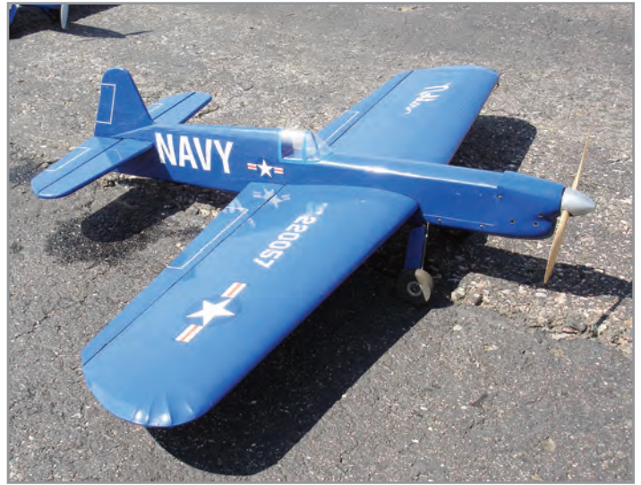
Mark Gerber's ARF Nobler features an Aero Tiger .36 for power. The Nobler met its demise during the contest going in hard on the nose after the motor quit unexpectedly. The motor fortunately seemed undamaged, saved, it appeared, by the collapsible "mystery wood" motor mounts that gave way under the impact. Pitcher photo.
