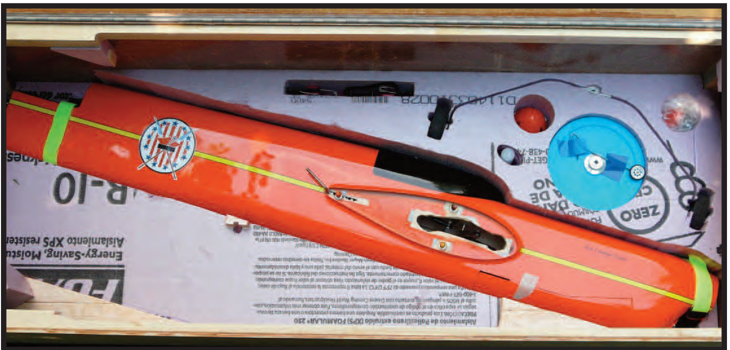
Howard's airplane fits into this wee box. A two-piece fuselage would have allowed more volume within the 62-inch-total-dimension airline constraint.
