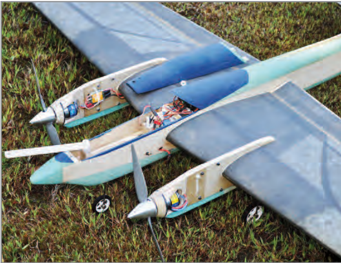
Bob Hunt and Bud Wieder brought their new twin-engine test-bed electric ship and flew a few demo flights with it. The ship also features retractable landing gear!
