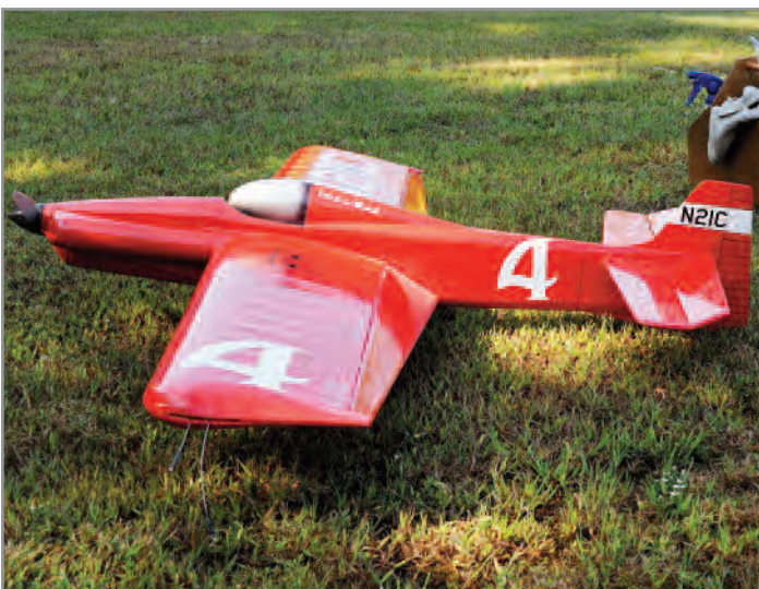
Jim Damerell's new, original-design, electric-powered Cosmic Wind features RC throttle control.
