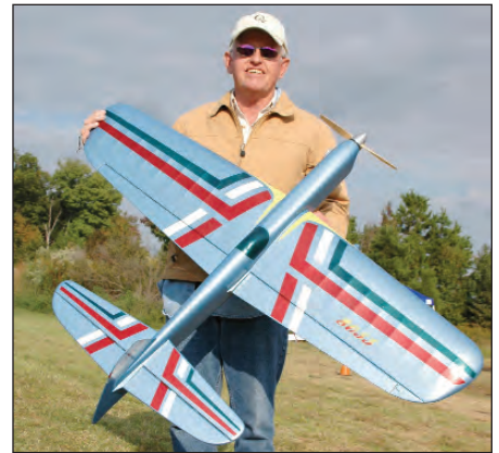
Eddie Ruane holding his Tempest 40. This plane is built around a Vector 40 wing, uses ST .46 for power, automotive paint finish. The ST power package handled the wind very well! Martine photo.
