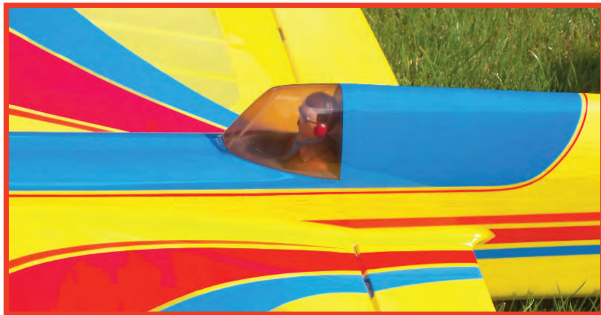
Here are the canopy and wing fillets on Pete's Rondinelli Venus.
