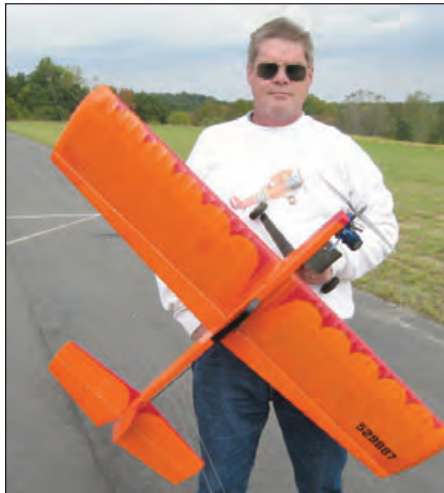
Clayton Berry with his original-design profile ship. Derived from Sig Twister, LA .46 power, Clayton used it for Profile and Expert at Huntersville.
